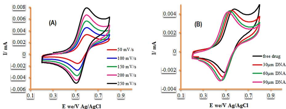
**Figure 2.** (A) Cyclic voltammograms of 2 mM compound (2F) at different scan rates. (B) Cyclic voltammograms of 2 mM compound (2F) in the absence and presence of 30  $\mu\text{M}$ , 60  $\mu\text{M}$  and 90  $\mu\text{M}$  DNA showing a decrease in  $I$  from  $I_0$  and a -ve shift in peak potential showing electrostatic interactions.
