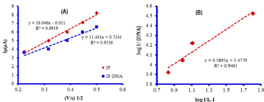
**Figure 3.** (A) Plots of  $I$  vs.  $v^{1/2}$ , for the determination of diffusion coefficients of compound 2F ( $0 \mu M$  DNA) and 2F-DNA. (B) Plot of  $\log (1/[DNA])$  vs  $\log (I/I_0 - I)$  for determination of binding constant
