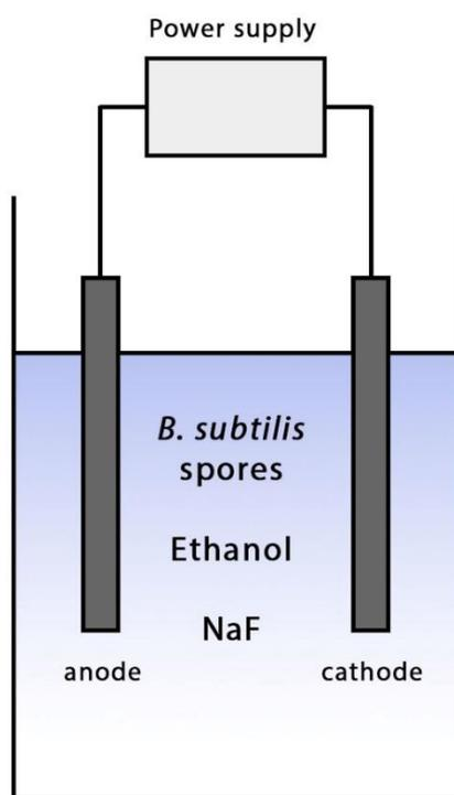
**Figure 1.** The electrochemical set-up reactor applied in this study
