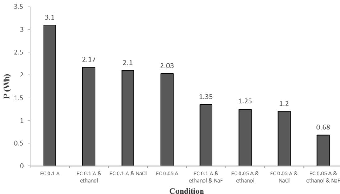
**Figure 6.** Measurement of the energy consumption of various current and electrolytes concentration ( $0.4 \text{ mol.L}^{-1}$  ethanol,  $4 \text{ mg.L}^{-1}$  NaCl,  $4 \text{ mg.L}^{-1}$  NaF) for  $10^3$  *B. subtilis* spores per mL removed from water.
