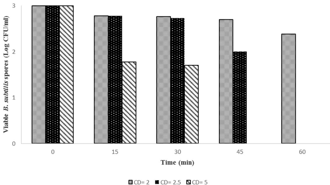
**Figure 4.** Inactivation of *B. subtilis* spores as a function of electrolysis time (min) and applied current density. Experimental conditions: batch mode,  $10^3 \text{ CFU}\cdot\text{mL}^{-1}$ , neutral pH,  $T = 25^\circ\text{C}$ , with applying  $0.4 \text{ mol}\cdot\text{L}^{-1}$  ethanol.
