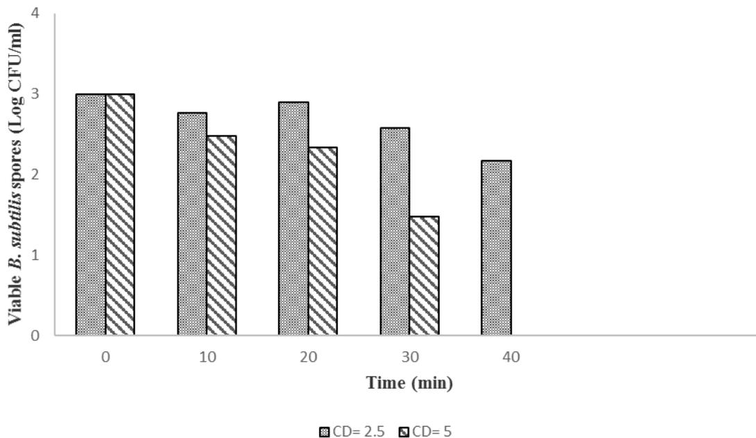
**Figure 5.** Inactivation of *B. subtilis* spores as a function of electrolysis time (min) and applied current density. Experimental conditions: batch mode,  $10^3$  CFU·mL<sup>-1</sup>, neutral pH, T = 25°C, with applying 0.4 mol·L<sup>-1</sup> ethanol and 4 mg·L<sup>-1</sup> NaF.
