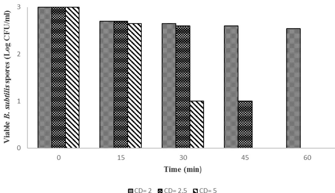
**Figure 3.** Inactivation of *B. subtilis* spores as a function of electrolysis time (min) and applied current density. Experimental conditions: batch mode, 10<sup>3</sup> CFU·mL<sup>-1</sup>, neutral pH, T = 25°C, with applying supporting electrolytes 4 mg·L<sup>-1</sup> NaCl.
