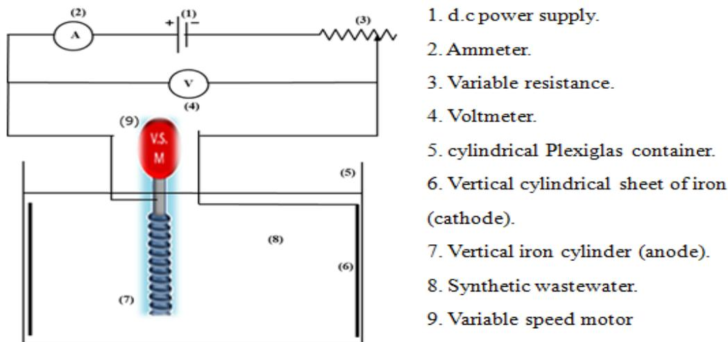
**Figure 1.** Experimental setup for the vertical anodes.
