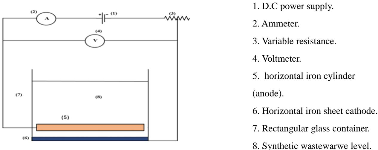
**Figure 2.** Experimental setup for the horizontal anodes.
