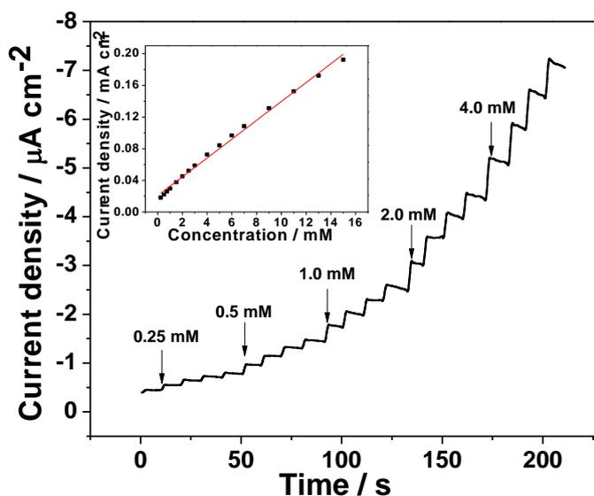
**Figure 5.** Amperometric response of the porous PtCu-EGN-IL/GCE to successive addition of ethanol. Support electrolyte: 0.5 M H<sub>2</sub>SO<sub>4</sub>; applied potential: 0.65 V. Inset: corresponding calibration curve.
