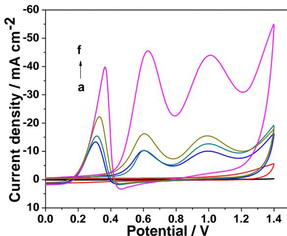
**Figure 4.** Cyclic voltammograms of GCE (a), EGN-IL/GCE(b), porous PtCu/GCE (c), Pt-EGN-IL/GCE (d), porous PtCu-EGN/GCE (e) and porous PtCu-EGN-IL/GCE (f) in 0.5 M H<sub>2</sub>SO<sub>4</sub> containing 0.5 M ethanol.
