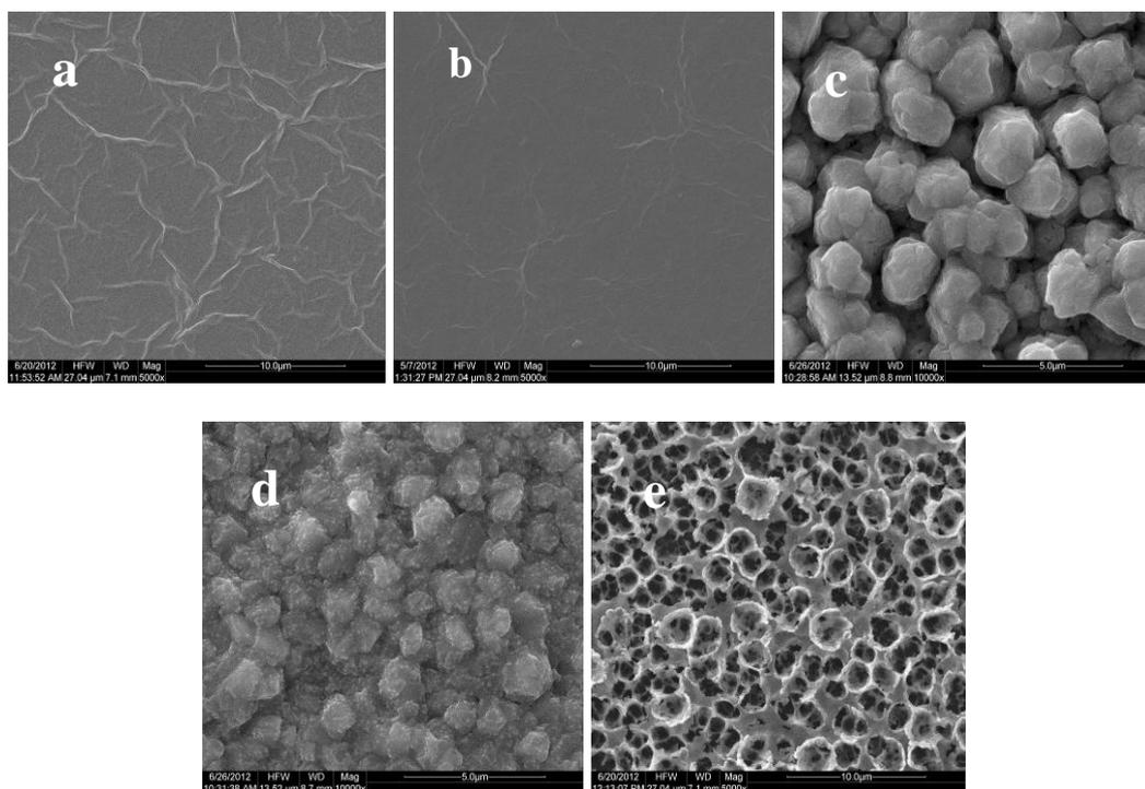
**Figure 1.** SEM images of EGN (a), EGN-IL/ITO (b), PtCu/ITO(c) , PtCu-EGN-IL/ITO (d) and porous PtCu-EGN-IL/ITO (e). The solution composition (for electrodeposition): 0.2 M  $\text{Na}_2\text{SO}_4$  + 1.0 mM  $\text{H}_2\text{Pt}_6\text{Cl}_4$  + 100 mM  $\text{CuSO}_4$ ; electrodeposition potential: -0.2 V; electrodeposition time: 500 s.
