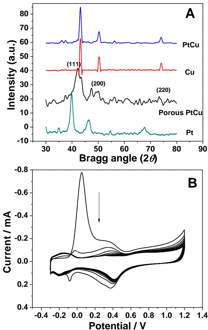
**Figure 2.** (A) XRD patterns of PtCu, Cu, porous PtCu and Pt (from upper to bottom) electrodeposited on EGN-IL film. (B) Cyclic voltammograms of PtCu-EGN-IL/GCE in 0.5 M H<sub>2</sub>SO<sub>4</sub> (from outer to inner: 1<sup>st</sup> CV to 10<sup>th</sup> CV). Scan rate: 100 mV s<sup>-1</sup>.
