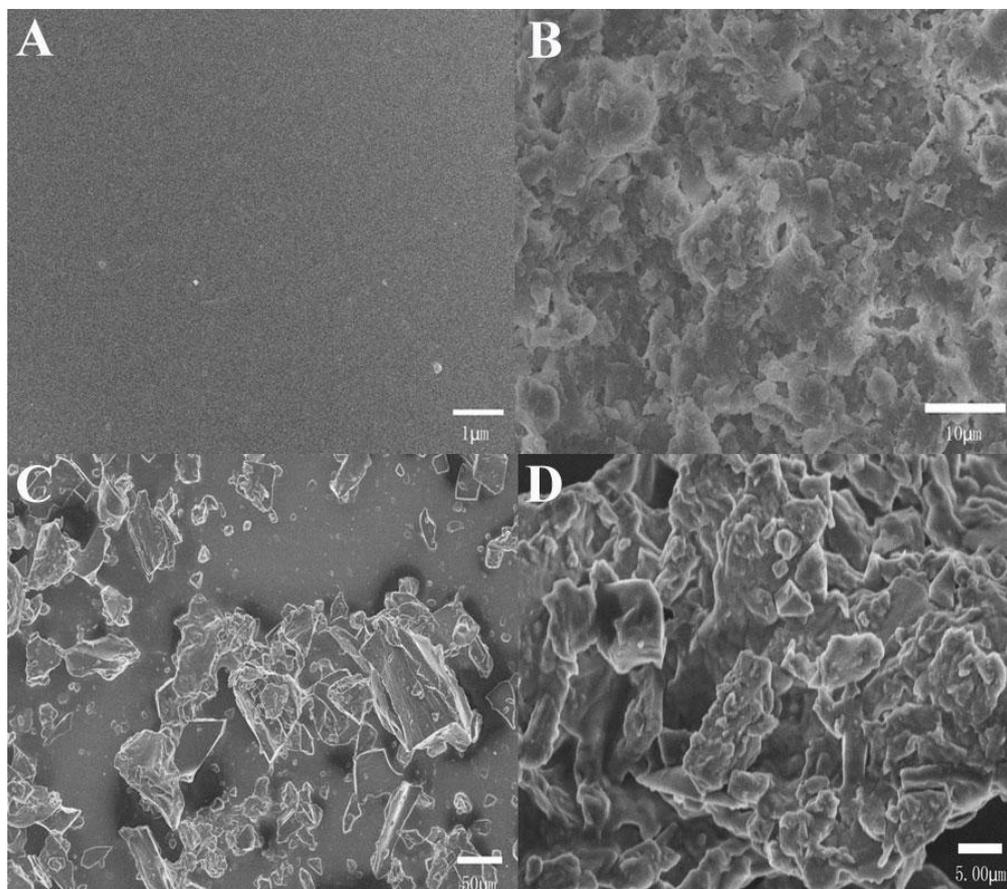
**Figure 2.** SEM images of CMC film (A, magnification, 10,000×), MMT film (B, magnification, 10,000×), and MMT-CMC-BC film (C, magnification, 2,000×, and D, magnification, 20,000×)
