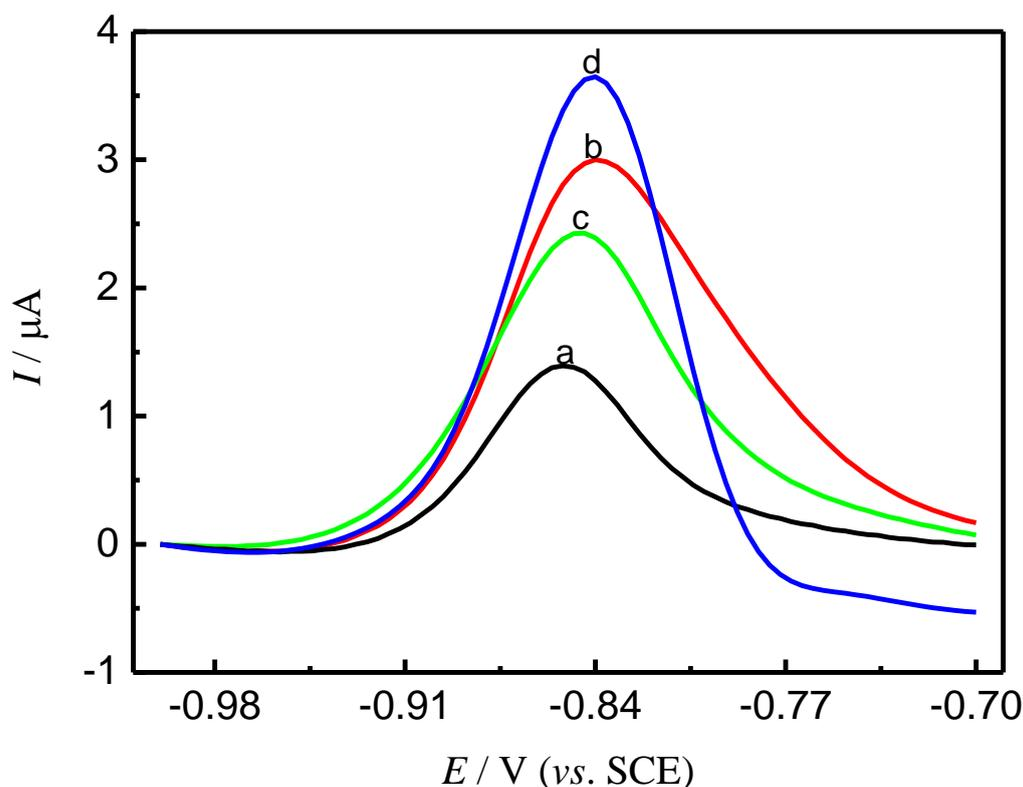
**Figure 6.** Effect of treatment methods on sensing performance for the SWASV detection of  $\text{Cd}^{2+}$ . Bare GCE (a), MMT-CMC-BC treated with nitric acid/GCE (b), MMT-CMC-BC treated with sodium hydroxide /GCE (c), MMT-CMC-BC/GCE (d).
