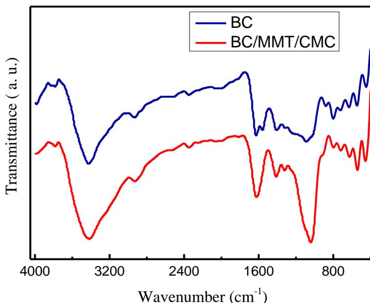
**Figure 3.** FT-IR spectra of BC and BC-CMC-MMT
