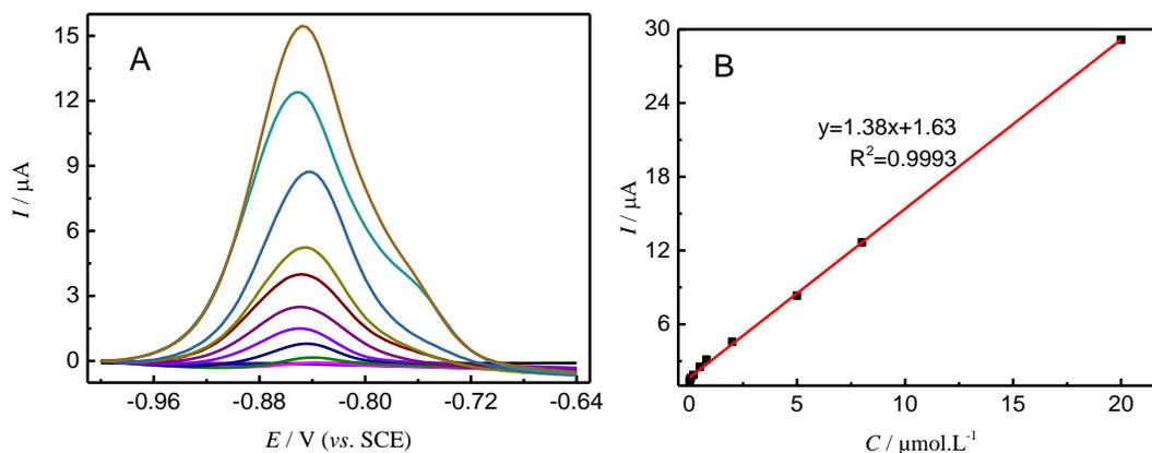
**Figure 10.** The stripping voltammograms of MMT-CMC-BC/GCE for  $\text{Cd}^{2+}$  detection in 0.1 M ABS (A), and plots of SWASV peak currents vs. corresponding  $\text{Cd}^{2+}$  concentrations (B).
