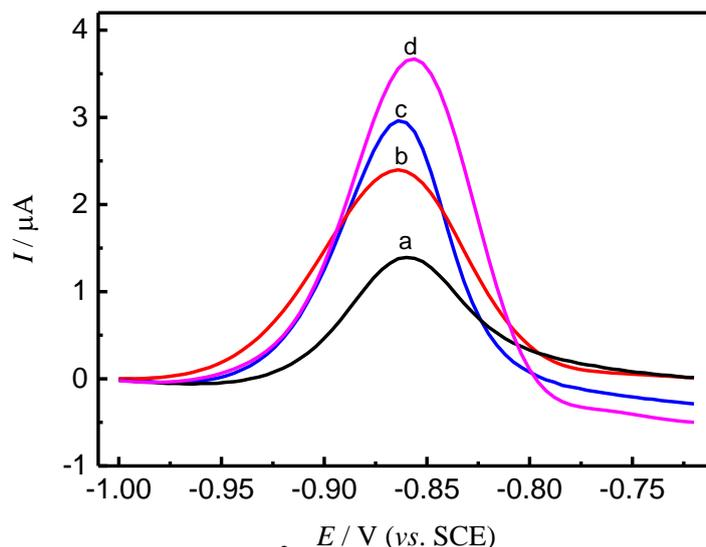
**Figure 4.** Electrochemical behaviors of  $\text{Cd}^{2+}$  in ABS at bare GCE (a), MMT-CMC/GCE (b), BC-CMC/GCE (c), and MMT-CMC-BC/GCE (d).
