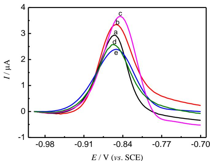
**Figure 5.** The effect of different ratios of both MMT and BC dispersed by CMC on sensing performance for the SWASV detection of  $\text{Cd}^{2+}$ . Different ratios of MMT and BC is 10:0 (a), 7:3 (b), 5:5 (c), 3:7 (d) and 0:10 (e).
