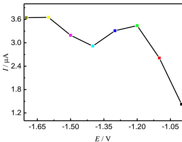
**Figure 8.** The effect of deposition potentials using SWASV in ABS containing 100 nM Cd<sup>2+</sup>.
