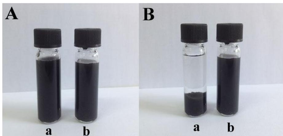
**Figure 1.** The photographs of BC (a) and MMT-CMC-BC (b) in water after ultrasonic oscillations, and the fresh prepared samples (A) and the sample after 5 days of stationary cultivation (B).
