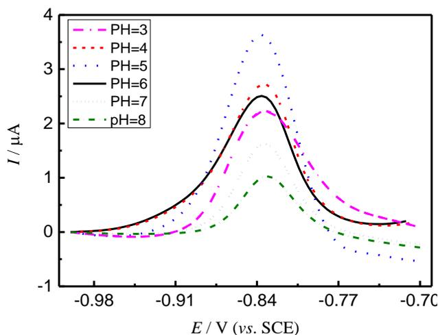
**Figure 7.** Effect of pH using SWASV in ABS containing 100 nM Cd<sup>2+</sup>.
