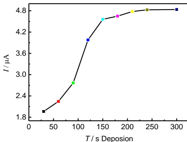
**Figure 9.** The effect of deposition time using SWASV in 0.1 M ABS (pH=5.0) containing of 100 nM  $\text{Cd}(\text{II})$ .
