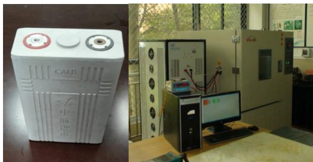
Figure 3. Test battery cell and test instrument
