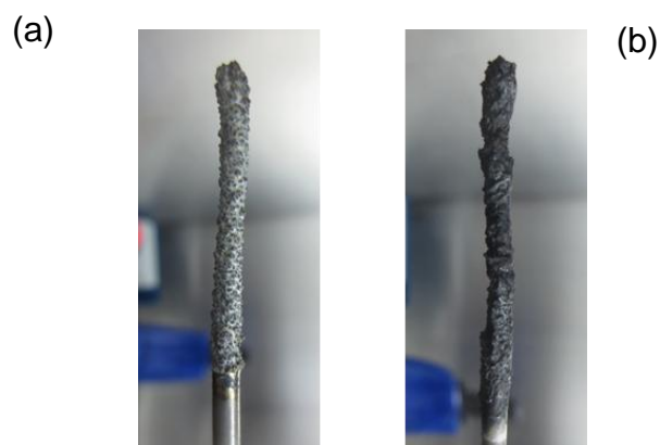
Figure 2. Photo images of Zr deposits electrorefined in (a) LiCl-KCl-0.07 M ZrCl 4 and (b) LiCl-KCl-0.07 M ZrF 4 . The applied potential was -1.1 V vs. Ag/Ag + .
