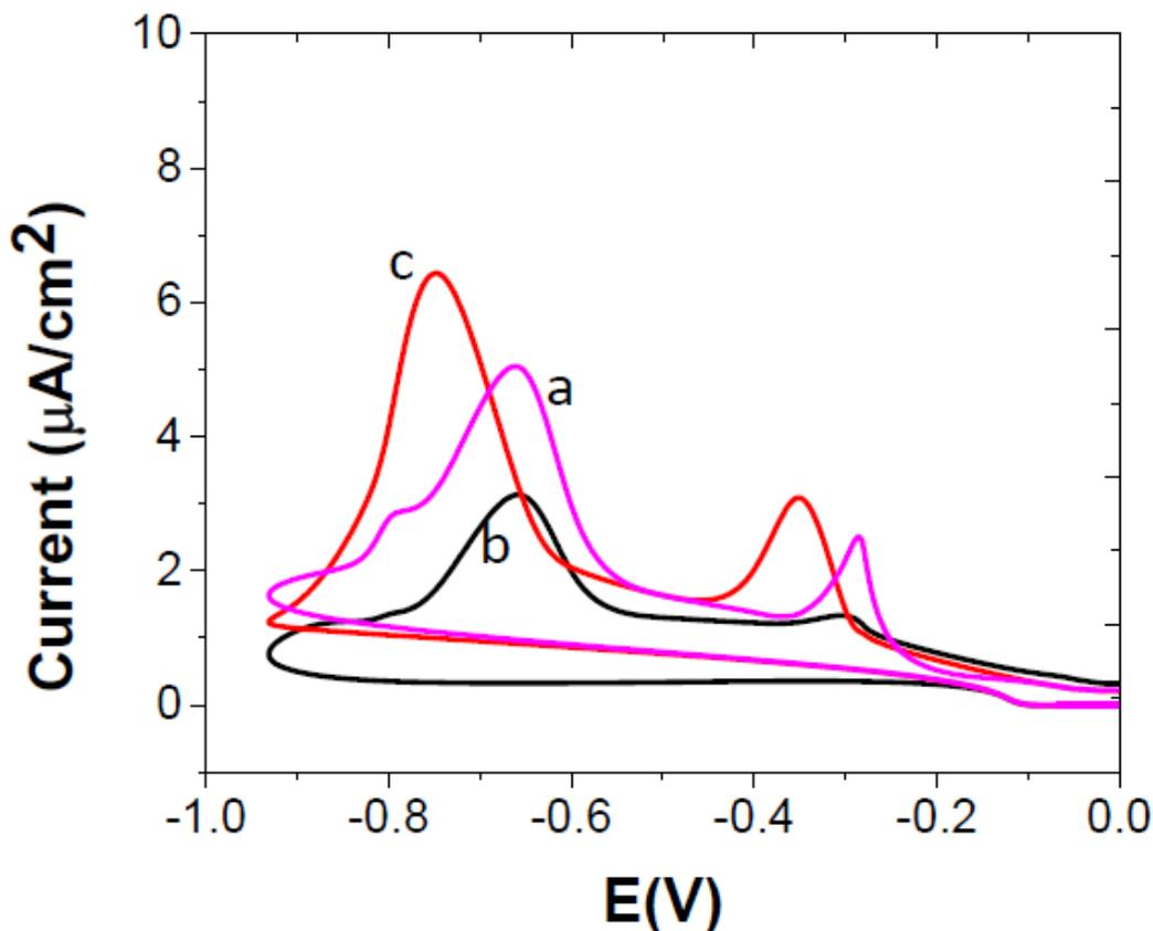
**Figure 3.** Cyclic voltammograms of DMV, NTF at bare GCE (a), CS/GCE (b) and RGO/CS/GCE (c), accumulation time: 100 s; pH: 6.0; accumulation potential: -0.32 V; scan rate: 20 mVs<sup>-1</sup>, concentration of OPs: 4.0 μg mL<sup>-1</sup>.
