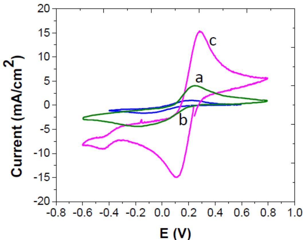
**Figure 2.** Typical cyclic voltammogram of bare GCE(a), CS/GCE (b) and RGO/CS/GCE (c) in 5.0 mM  $[\text{Fe}(\text{CN})_6]^{3-/4-}$  containing 0.1 M KCl at  $20 \text{ mV s}^{-1}$ , at pH 6.0, accumulation time: 100 s; accumulation potential:  $-0.32\text{V}$ ; concentration of OPs:  $4.0 \mu\text{g mL}^{-1}$ .
