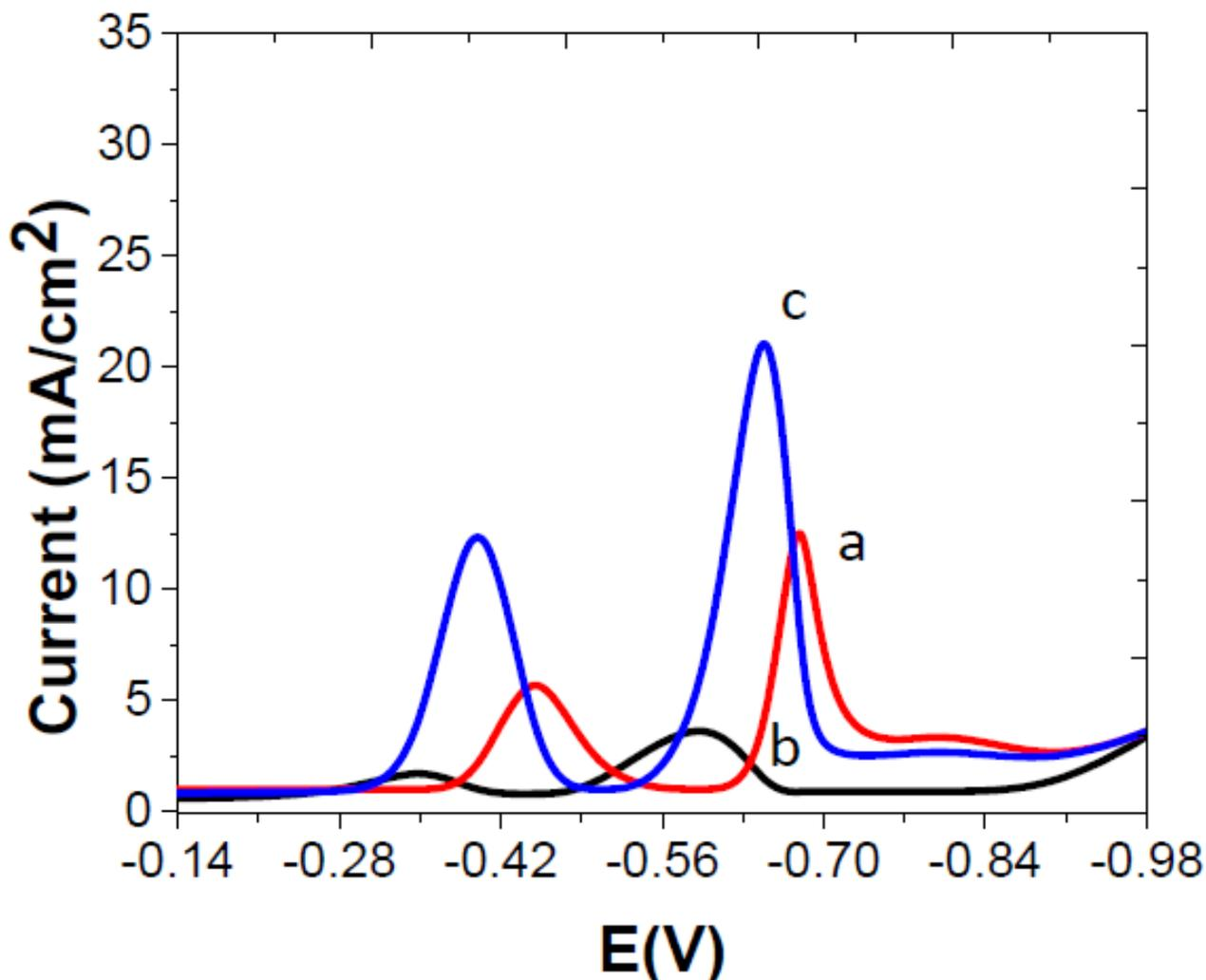
**Figure 4.** Square wave voltammograms of DMV and NTF at bare GCE (a), CS/GCE (b) and RGO/CS/GCE (c), accumulation time: 100 s; pH: 6.0; accumulation potential: -0.32 V; scan rate:  $20 \text{ mVs}^{-1}$ , square wave frequency 60 Hz; pulse amplitude 50mV; concentration of OPs:  $4.0 \mu\text{g mL}^{-1}$ .
