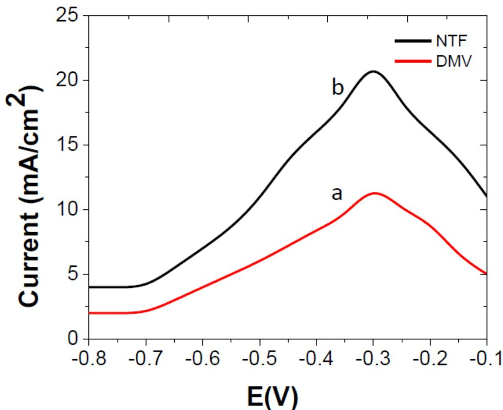
**Figure 6.** Effect of accumulation potential on the square wave voltammetry of DMV (a) and NTF (b) at pH 6.0, concentration of OPs:  $4.0 \mu\text{g mL}^{-1}$ ; accumulation time: 100 sec; square wave frequency 60 Hz; pulse amplitude 50mV; scan rate:  $20 \text{ mV s}^{-1}$ .
