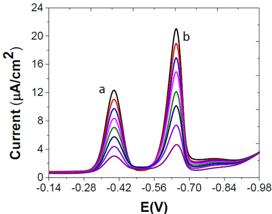
**Figure 8.** Square wave voltammetry responses of RGO/CS/GCE in a BR buffer at pH 6.0 after incubation with 0.2 (a), 4.0 (b), 8.0 (c), 12.0 (d), 16.0 (e), 20.0 (f), 24.0 (g), 30.0 (h)  $\mu\text{g mL}^{-1}$  of DMV (a) and NTF (b), accumulation potential: -0.32 V; square wave frequency 60 Hz; pulse amplitude 50mV; scan rate: 20  $\text{mV s}^{-1}$ .
