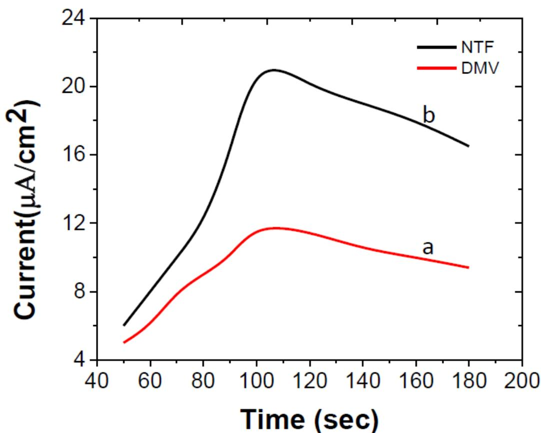
**Figure 7.** Effect of accumulation time on the square wave voltammetry of DMV(a) and NTF (b) at pH 6.0, concentration of OPs:  $4.0 \mu\text{g mL}^{-1}$ ; accumulation potential:  $-0.32 \text{ V}$ ; square wave frequency 60 Hz; pulse amplitude 50mV; scan rate:  $20 \text{ mV s}^{-1}$ .
