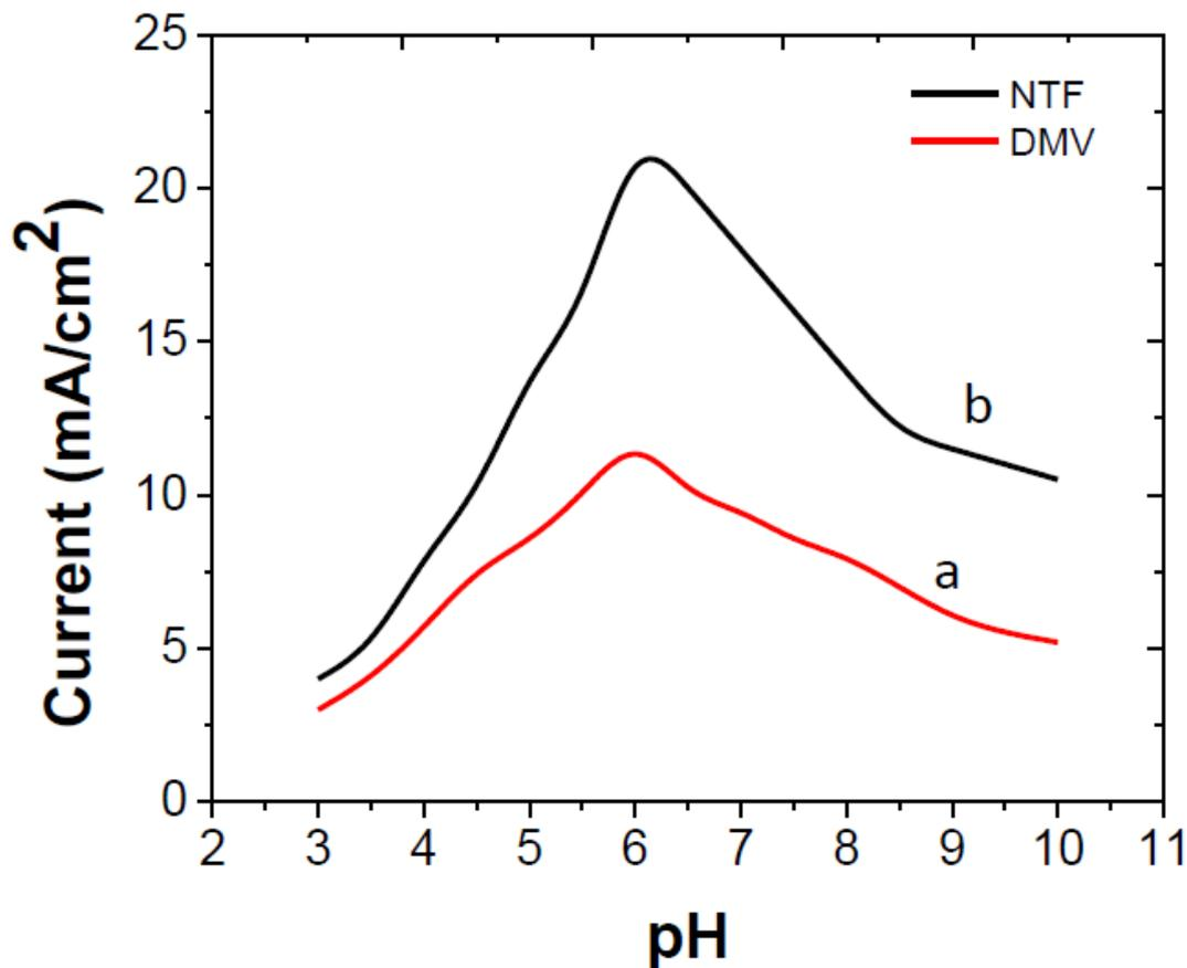
**Figure 5.** Effect of pH on DMV (a) and NTF (b) solution at RGO/CS/GCE, accumulation time: 100 s.; accumulation potential: -0.32V; square wave frequency 60 Hz; pulse amplitude 50mV; concentration of OPs:  $4.0 \mu\text{g mL}^{-1}$ , scan rate:  $20 \text{ mVs}^{-1}$ .
