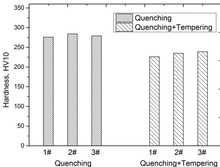
**Figure 1.** Hardness of the 12MnNiVR steel with two different heat treatments
