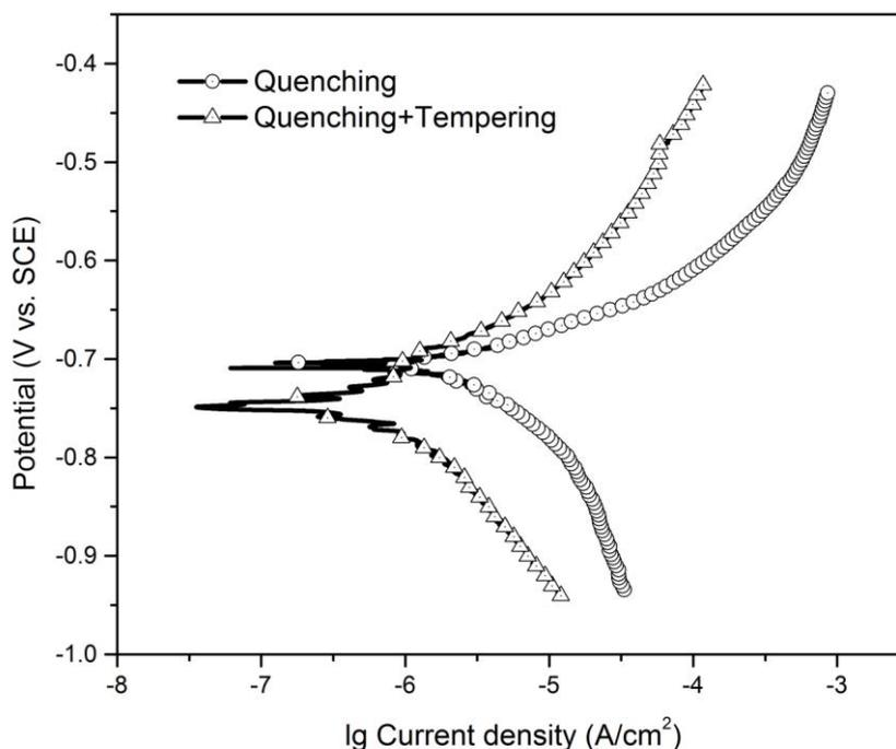
**Figure 4.** Polarization curves of the 12MnNiVR steel with two kinds of heat treatments in 3.5 wt% NaCl solution. The polarization scanning rate was 0.2 mV/s. All tests were performed at room temperature and atmosphere.
