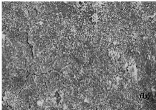
**Figure 3.** SEM images showing the corrosion scales that formed on the 12MnNiVR steel with two different heat treatments: (a) Quenching; (b) Quenching + Tempering
