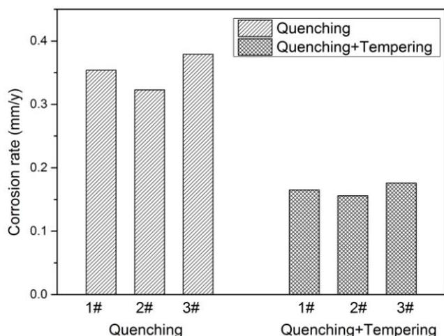
**Figure 2.** Corrosion rates of the 12MnNiVR steel with two different heat treatments
