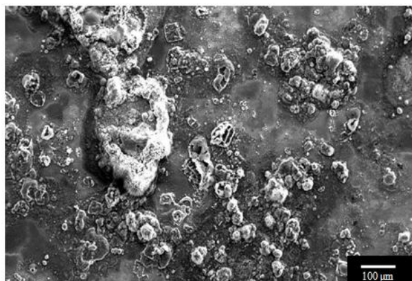
Figure 4. The morphology on the zinc sample covered by 200 μg cm -2 NaCl particles at 75% RH and 25 °C after 168 h of exposure.
