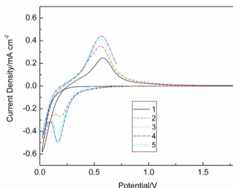
**Figure 5.** Cyclic voltammetry of Si NWs electrode with a scan rate of 0.05mV/s of the first 5 cycles
