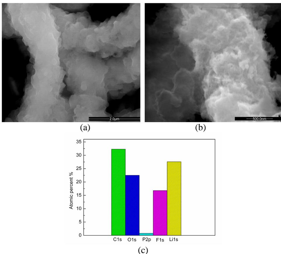
**Figure 6.** (a) and (b) SEM images of Si NWs electrode after cycling, (c) Atomic percent of SEI film on Si NWs electrode characterized by XPS
