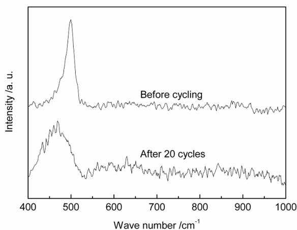
**Figure 2.** Raman shifts of as-prepared silicon nanowires before and after 20 cycles
