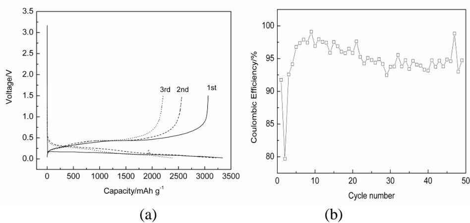
**Figure 4.** (a) The charge-discharge profile of silicon NWs anode for the first three cycles. (b) The Coulombic efficiency of the Si NWs anode vs cycle number
