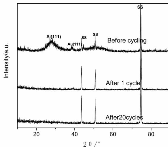
**Figure 3.** The XRD profiles of as-prepared silicon nanowires before and after cycling
