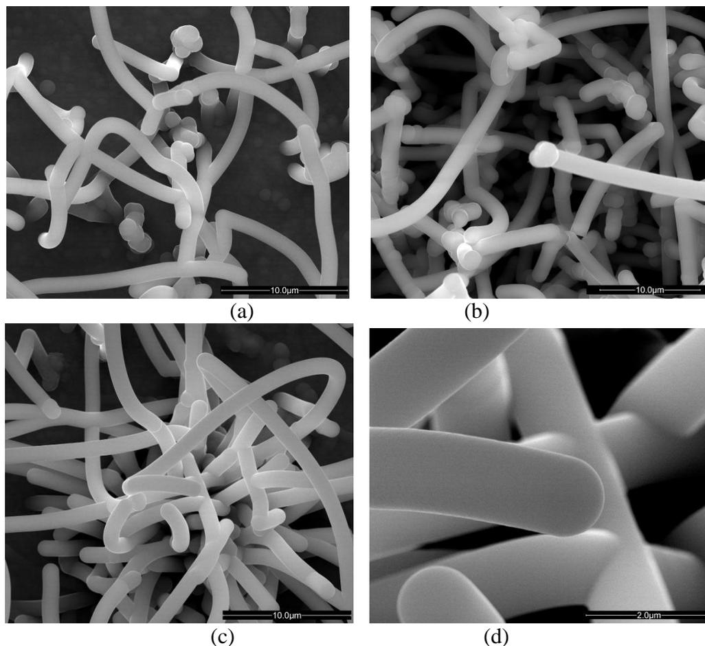
**Figure 1.** The SEM images of silicon nanowires deposited with different time: (a) 2min, (b) 5min, (c) and (d) 30min
