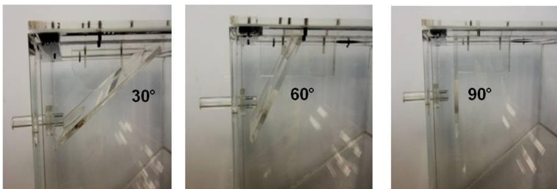
Figure 4. Shock plates positioned at different impingement angles of inclination (a) 30°, (b) 60° and (c) 90°.
