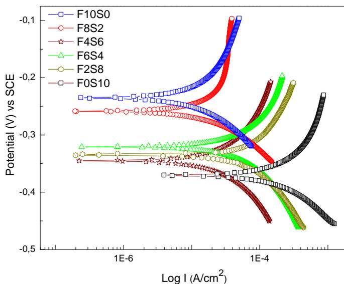
**Figure 3.** Polarization curves where it represents the electrochemical behaviour of concrete evaluated.
