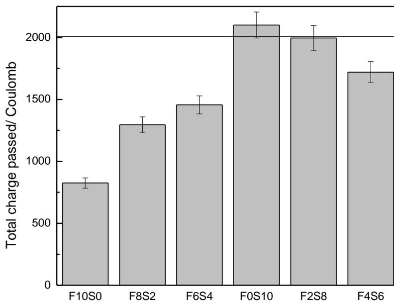
**Figure 1.** Ionic charge of alternative cements and binary mixtures.
