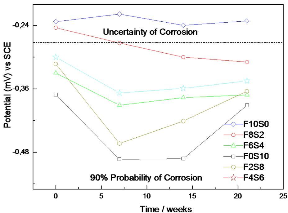
**Figure 2.** Half-cell potential values versus time for steel rebars embedded in mixtures of fly ash and steel slag. Evaluation by 21 weeks.
