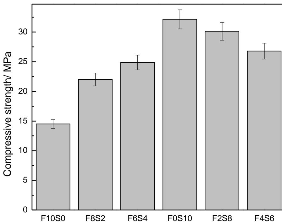
**Figure 4.** Compressive strength alternative concrete based on fly ash and steel slag and evaluated at 28 days.
