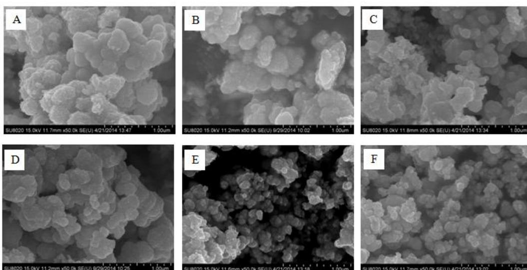
**Figure 8.** Surface morphology of electrodeposited Pd from [emim]OTf at the current densities of  $0.010 \text{ mA/mm}^2$  (A),  $0.013 \text{ mA/mm}^2$  (B),  $0.017 \text{ mA/mm}^2$  (C),  $0.020 \text{ mA/mm}^2$  (D),  $0.023 \text{ mA/mm}^2$  (E), and  $0.027 \text{ mA/mm}^2$  (F).
