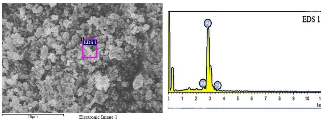
**Figure 2.** Surface morphology and EDS pattern of the Pd deposits from [emim]OTf taken by galvanostatic electrodeposition.
