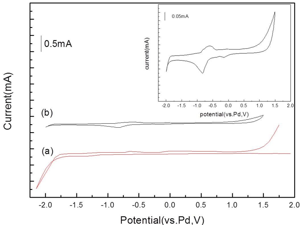
**Figure 1.** Electrochemical window of [emim]OTf (a) and cyclic voltammograms of Pd (II) chloride in [emim]OTf (b). T=298K; Scan rate: 50mV/s; Working and counter electrodes: Pt wire; Reference electrode: Pd wire; Mole ratio of [emim]OTf and PdCl<sub>2</sub>: 45:1.
