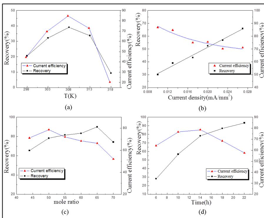
Figure 7. Effect of temperature (a), current density (b), mole ratio (c), and electrolysis time (d) on current efficiency and recovery of electrodeposited Pd.
