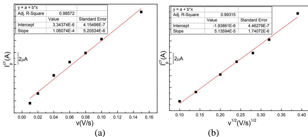
**Figure 5.** Relationship between cathodic peak current  $I_p^{c1}$  and v (a) or  $v^{1/2}$  (b) for the reduction of Pd (II) at 303K.
