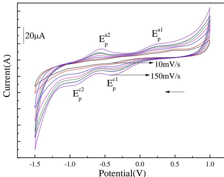
**Figure 4.** Cyclic voltammograms of a solution of 12mM PdCl<sub>2</sub> in [emim]OTf at various sweeping rates at 303K. Working and counter electrodes: Pt wire; Reference electrode: Pd wire. Sweeping rates (mV s<sup>-1</sup>): (a) 10, (b) 20, (c) 40, (d) 60, (e) 80, (f) 100, and (g) 150.
