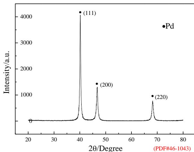
**Figure 3.** XRD pattern of the depositions obtained by electrolysis of [emim]OTf-PdCl<sub>2</sub>.
