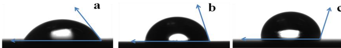
Figure 1. Sessile water drop images on: (a) Bare aluminum alloy; (b) The sample treated in \text{Ce}(\text{NO}_3)_3 solution; (c) The sample treated in \text{Ce}(\text{NO}_3)_3\text{-H}_2\text{O}_2 solution.
