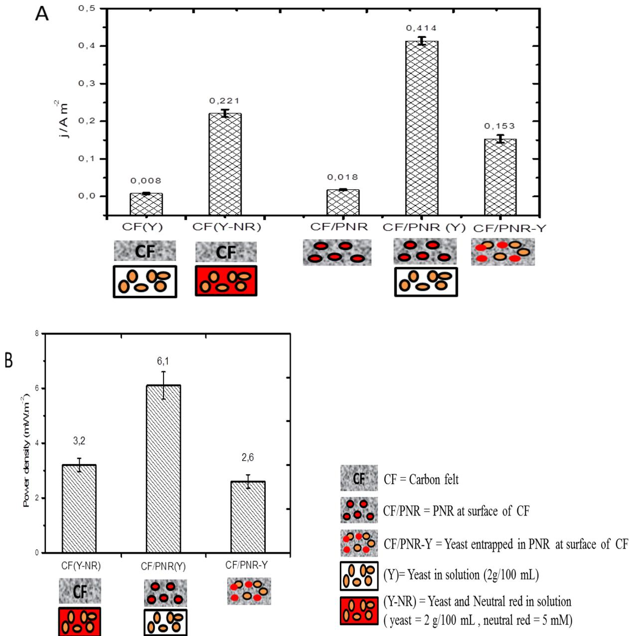
**Figure 7.** (A) Current density generated by the different anodes in a 0.1 M glucose solution and (B) Power density delivered at MFC.
