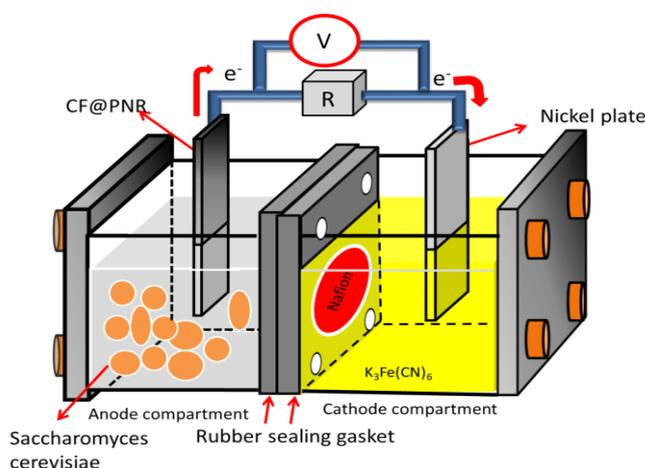
**Figure 1.** Scheme of the Microbial Fuel Cell (MFC) system
