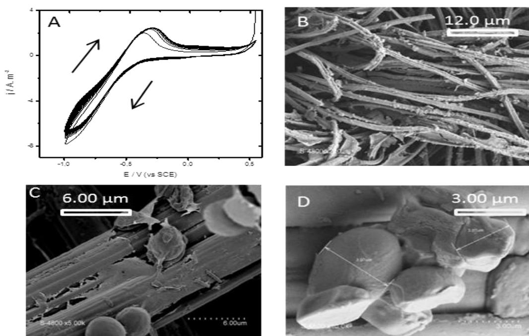
**Figure 4.** (A) Cyclic voltammogram of yeast entrapped in the PNR film (CF/PNR-Y) (15 cycles) and (B- to D) SEM images of the CF/PNR-Y membranes. Yeast was identified as cylindrical forms of around 3 microns of diameter.
