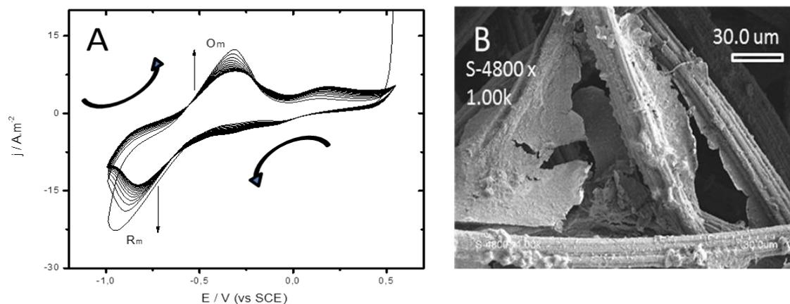
**Figure 2.** (A) Cyclic voltammogram of PNR (15 scans) and (B) SEM image of the CF/PNR membrane.
