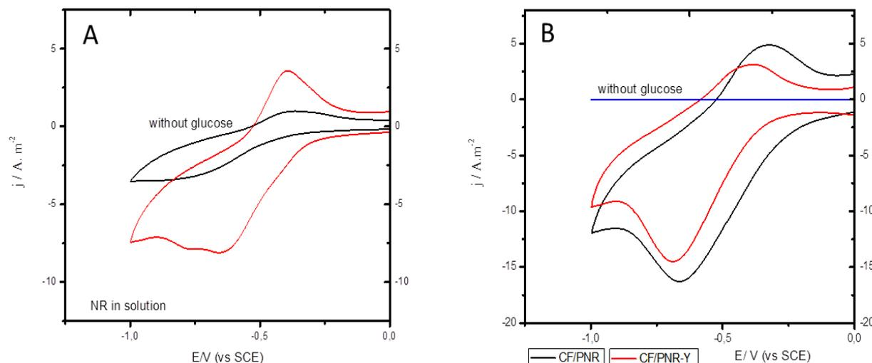
**Figure 6.** (A) Cyclic voltammogram at CF electrode in NR (5 mM), yeast (2 g/100 mL) in PB pH 6, without glucose (black line) and with glucose (0.1 M) (red line) and (B) at CF/PNR(Y) electrode (red line) and at CF/PNR electrode (black line) in NR (5 mM) in PB pH 6, with glucose (0.1 M): Red line: yeast at 2 g/100 mL, black line: yeast immobilized at electrode.
