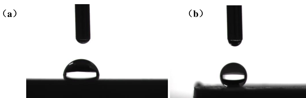
Figure 7. Shape of water drops placed on brass surface. (a) Self-assemble surface without anodization; (b) Self-assemble surface with anodization
