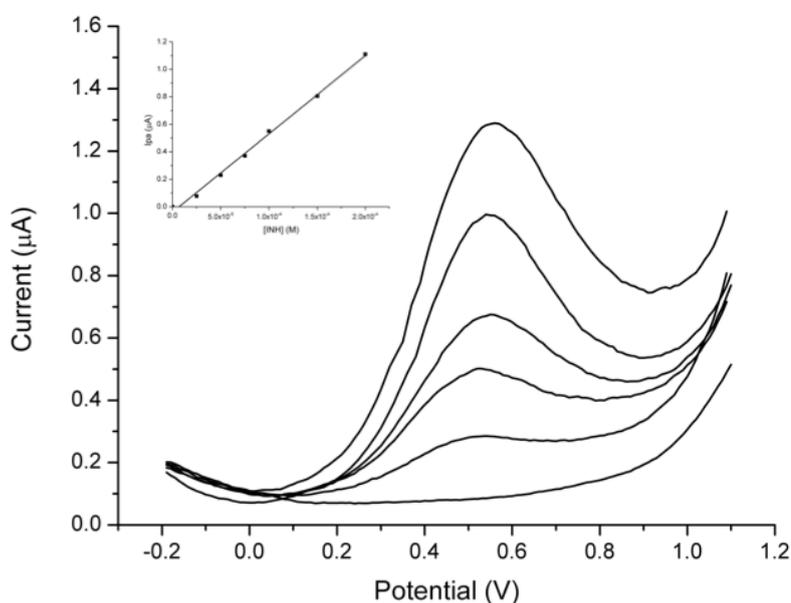
**Figure 5.** Square wave voltammograms obtained at under optimized conditions in 0.1 M PBS pH 7.0 containing 0.0,  $2.5 \times 10^{-5}$ ,  $5.0 \times 10^{-5}$ ,  $7.5 \times 10^{-5}$ ,  $1.0 \times 10^{-4}$ ,  $1.5 \times 10^{-4}$  M of INH. Inset: Analytical curve.
