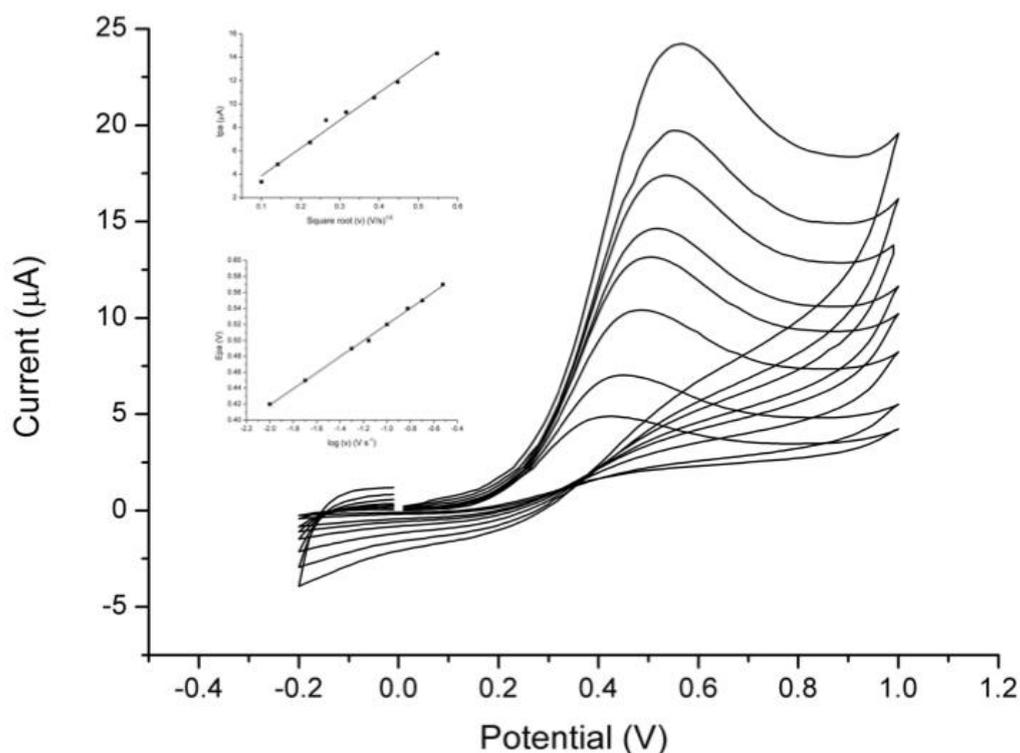
**Figure 4.** Cyclic voltammograms of a  $6.0 \times 10^{-5}$  M INH solution in PBS pH 7.0 at the Nafion-SPCE at different scan rates: 0.01, 0.02, 0.05, 0.07, 0.1, 0.15, 0.2 and 0.25  $\text{V s}^{-1}$ . Inset A: linear relationship between the peak currents and the square root of the scan rates. Inset B: linear relationship between the peak potentials and the logarithm of the scan rates.
