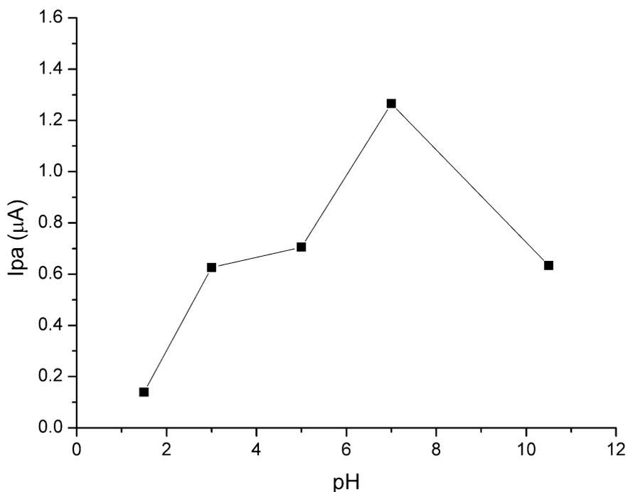
**Figure 1.** Plot of  $I_{pa}$  vs. pH obtained by SWV of a  $4.0 \times 10^{-5}$  M INH solution in 0.1 M PBS at different pH values: 1.5, 3.0, 5.0, 7.0 and 10.5 at the surface of unmodified SPCEs. Frequency: 10 Hz.
