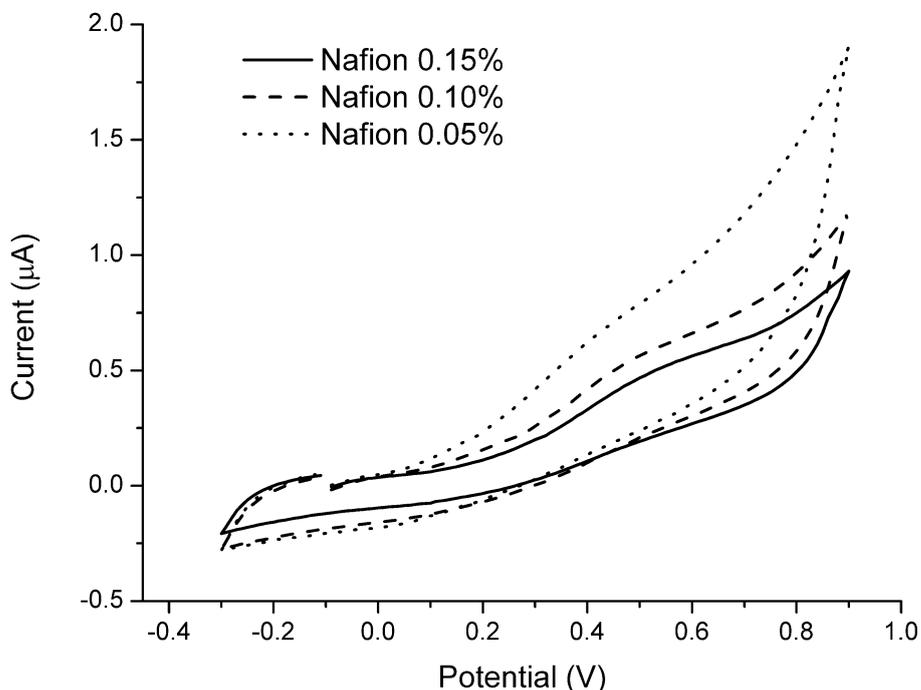
**Figure 2.** Cyclic voltammograms of a  $6.0 \times 10^{-5}$  M INH solution in PBS pH 7.0 at SPCEs modified with 0.15%, 0.10% and 0.05% Nafion solutions. Scan rate:  $0.10 \text{ V s}^{-1}$ .
