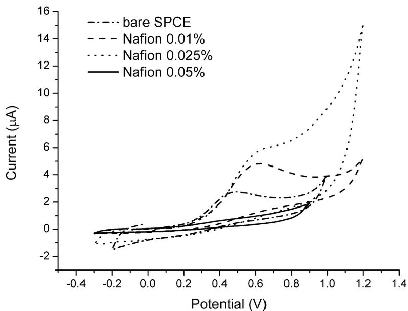
**Figure 3.** Cyclic voltammograms of a  $6.0 \times 10^{-5}$  M INH solution in PBS pH 7.0 at bare SPCE and SPCEs modified with 0.01%, 0.025% and 0.05% Nafion solutions. Scan rate:  $0.10 \text{ V s}^{-1}$ .
