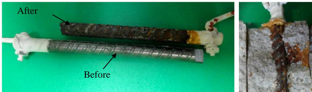
**Figure 11.** Reinforcement steel after ACTIV.
