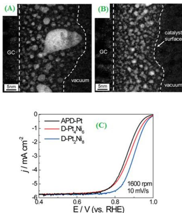
**Figure 5.** Cross-sectional HAADF-STEM images of  $\text{Pt}_2\text{Ni}_8$  (as-prepared) (A) and D- $\text{Pt}_2\text{Ni}_8$  (de-alloyed) (B) on glassy carbon substrates. (C) Linear-sweep voltammograms for the ORR of D- $\text{Pt}_4\text{Ni}_6$ , D- $\text{Pt}_2\text{Ni}_8$  and APD-Pt. ("Reprinted with permission from (ACS Catal. 5 (2015) 2209-2212). Copyright (2015) American Chemical Society").
