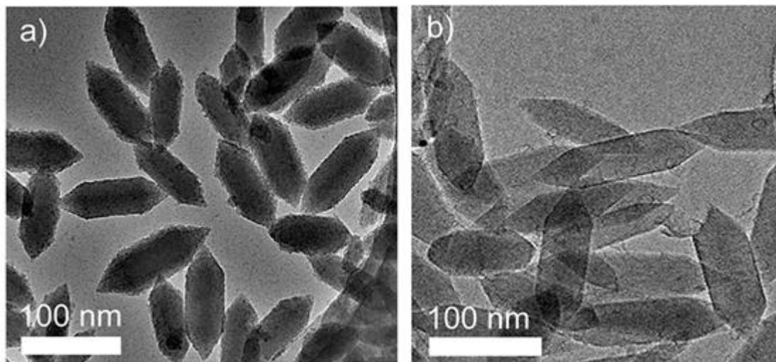
**Figure 1.** Shows (a and b) TEM images of nanoscale MIL-88B-NH<sub>3</sub> and CNPs. ("Reprinted with permission from (*ACS Nano* 8 (2014) 12660-12668). Copyright (2014) American Chemical Society").
