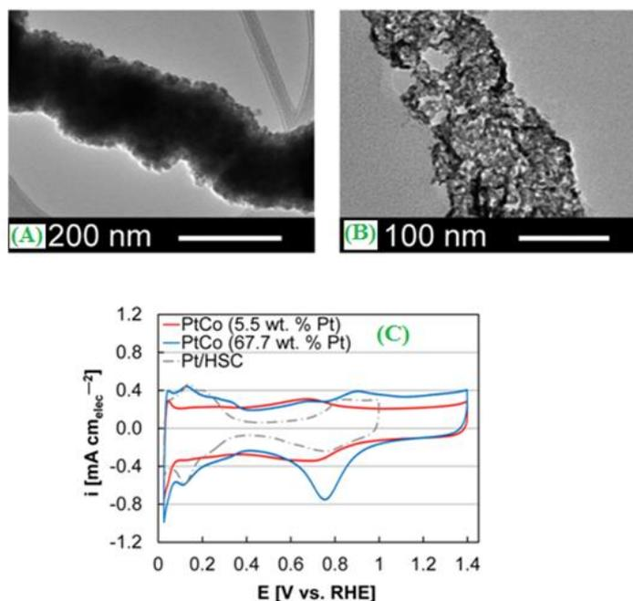
**Figure 9.** TEM images of PtCoNWs (21.1 wt % Pt): (A) as-synthesized, (B) following electrochemical break-in (C) Cyclic voltammograms curves of PtCoNWs (5.5 and 67.7 wt % Pt with graphitized carbon nanofibers, 60 wt %, added to catalyst inks) and Pt/HSC. ("Reprinted with permission from (ACS Catal. 4 (2014) 2680-2686). Copyright (2014) American Chemical Society").
