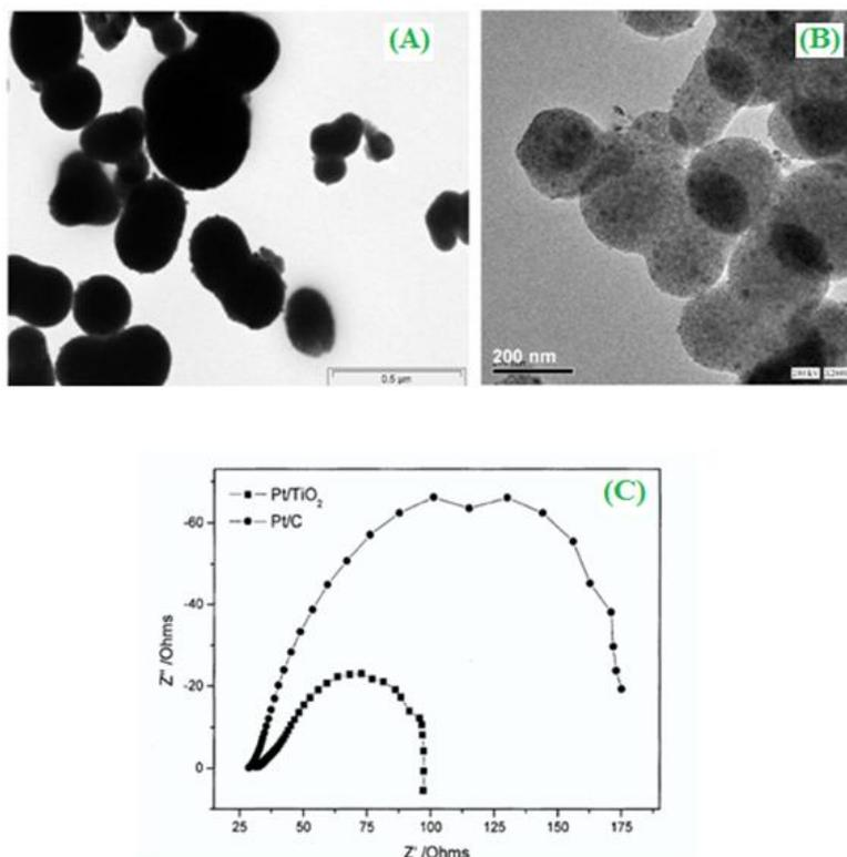
**Figure 12.** TEM images of (A) TiO<sub>2</sub> and (B) Pt/TiO<sub>2</sub> (C) Nyquist plot for the electrodes (Pt/TiO<sub>2</sub> and Pt/C) in 0.5 M H<sub>2</sub>SO<sub>4</sub> at open circuit potential. ("Reprinted with permission from (*J. Phys. Chem. C* 113 (2009) 18707-18712). Copyright (2009) American Chemical Society").
