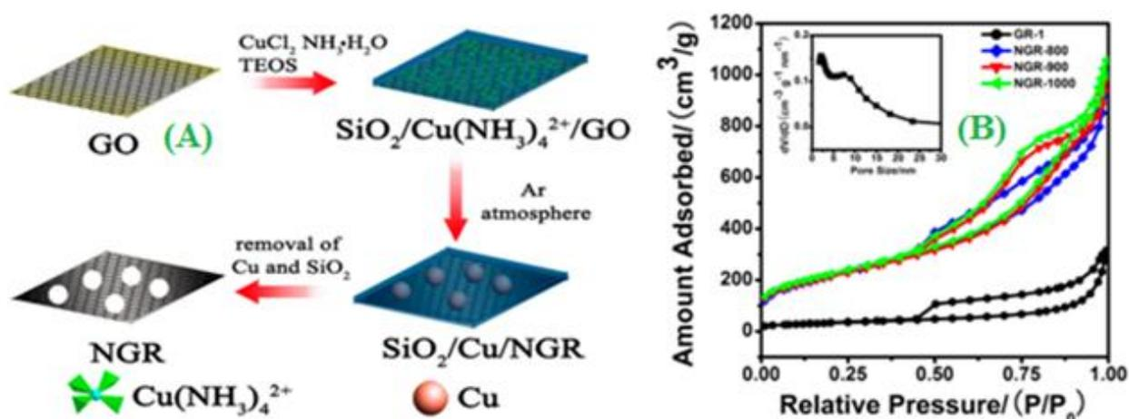
**Figure 6.** (A) Preparation Pathway of NGR (B) Nitrogen adsorption-desorption isotherms of NGR-800, NGR-900, NGR-1000, and GR-1. Inset: Pore size distribution of NGR-900. ("Reprinted with permission from (*ACS. Appl. Mater. Interfaces* 6 (2014) 3023-3030). Copyright (2014) American Chemical Society").
