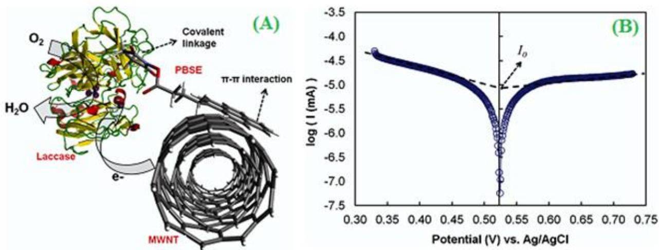
**Figure 11.** (A) Schematic of the bio-nanocomposite where laccase is tethered to MWNT using pyrenebutanoic acid succinimidyl ester (PBSE). (B) Linear sweep voltammograms showing Tafel regions at no rotation for the laccase-MWNT in phosphate buffer (pH 5.8). The applied potential range was from 0.33 to 0.73 V. ("Reprinted with permission from (*ACS Catal.* 2 (2012) 38-44). Copyright (2012) American Chemical Society").
