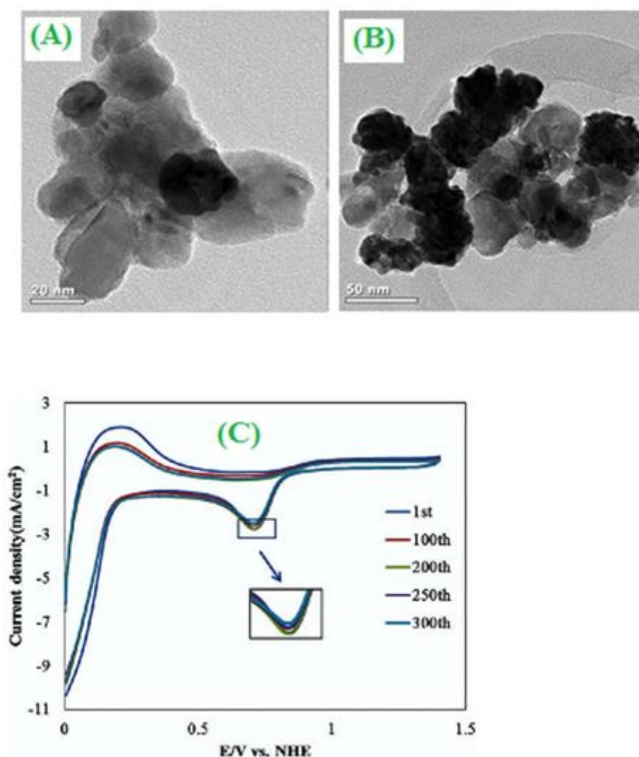
**Figure 4.** TEM (A) low (B) high images of Pt/WO<sub>3</sub> after cycling between 0 and 1.4 V 300 times. (C) Cyclic voltammograms of Pt/WO<sub>3</sub> in O<sub>2</sub> saturated 0.1 M HClO<sub>4</sub> between 0 and 1.4 V for 300 cycles; scan rate is 10 mV s<sup>-1</sup>. ("Reprinted with permission from (*ACS Catal.* 2 (2012) 456-463). Copyright (2012) American Chemical Society").
