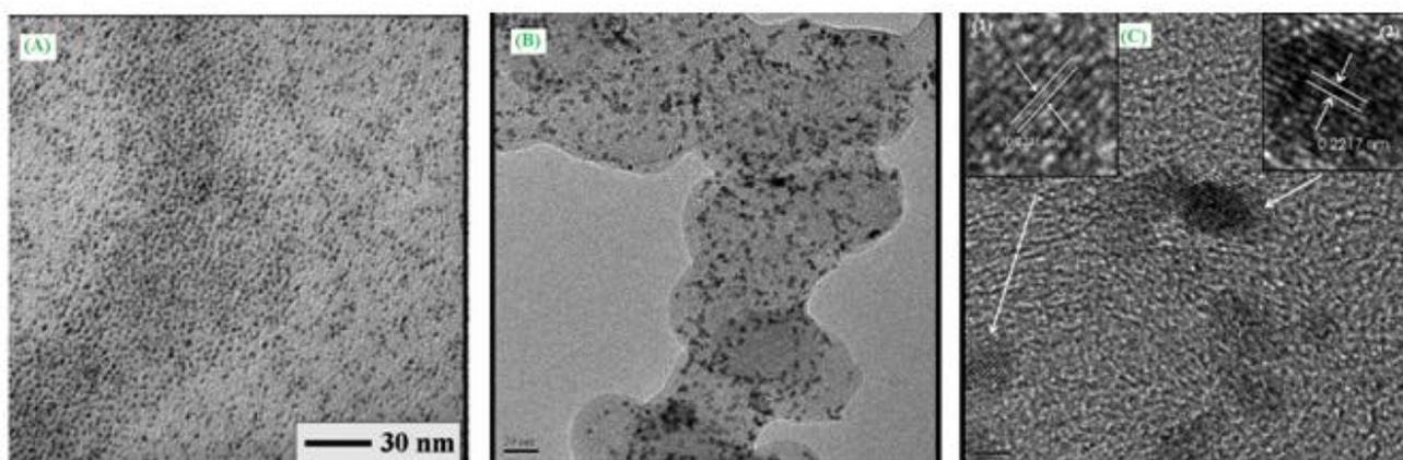
**Figure 7.** (A) TEM for a sample of as-synthesized  $\text{Pt}_{25}\text{Ir}_{20}\text{Co}_{55}$  nanoparticles ( $2.2 \pm 0.2 \text{ nm}$ ). (B) TEM (scale bar = 20 nm) and (C) HR-TEM (scale bar = 2 nm) for a sample of  $\text{Pt}_{25}\text{Ir}_{20}\text{Co}_{55}/\text{C}$  catalyst treated at  $400^\circ \text{C}$ . Inset: lattice fringes of (111) for the supported nanoparticles. ("Reprinted with permission from (*ACS Catal.* 1 (2011) 562-572). Copyright (2011) American Chemical Society").
