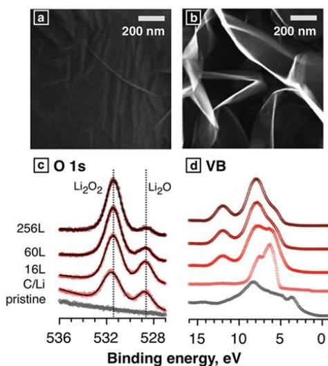
**Figure 3.** Top-view SEM images of the MLG (a) and CNW (b) samples. (c, d) O 1s and valence band photoemission spectra of pristine CNWs, lithiated CNWs, and the same sample during oxygen exposure. ("Reprinted with permission from (*ACS Nano* 9 (2015) 320-326). Copyright (2015) American Chemical Society").
