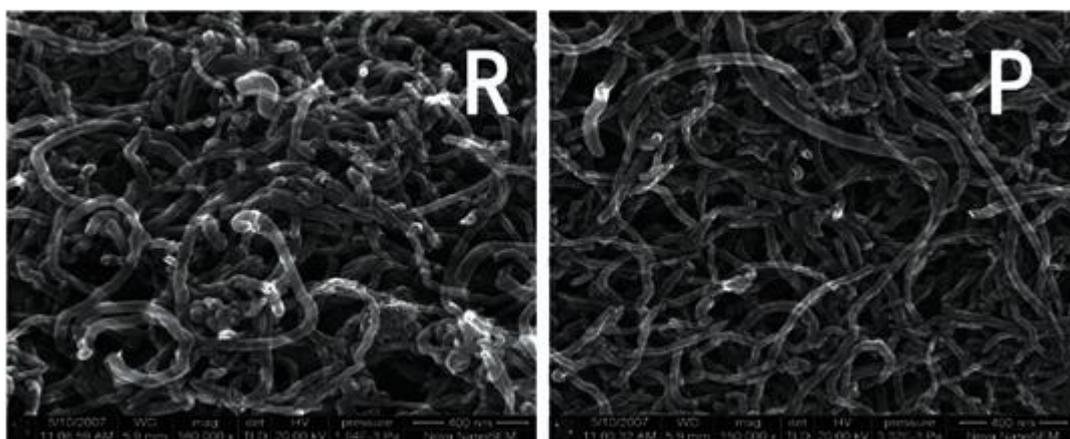
**Figure 2.** SEM images of *r*MCNTs (R) and *p*MCNTs (P). ("Reprinted with permission from (*J. Phys. Chem. C* 112 (2008) 2671-2677). Copyright (2008) American Chemical Society").
