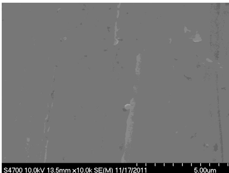
**Figure 1.** The surface morphology of the sample after fluorine PIII
