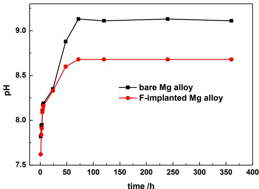
**Figure 3.** Change of pH values of bare and F-implanted Mg alloy in SBF
