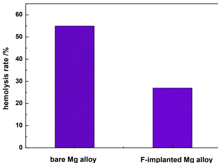
**Figure 5.** Hemolysis tests of bare and F-implanted Mg alloys
