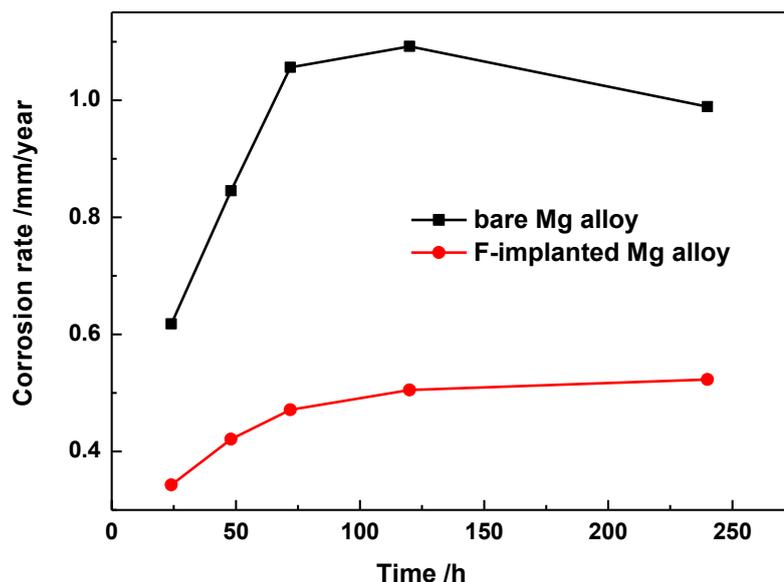
**Figure 4.** Corrosion rate of bare and F-implanted Mg alloy versus immersion time in the SBF
