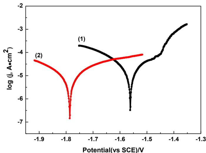
**Figure 2.** Potentiodynamic polarization behavior of (1) bare sample (2) F-implanted sample in the SBF
