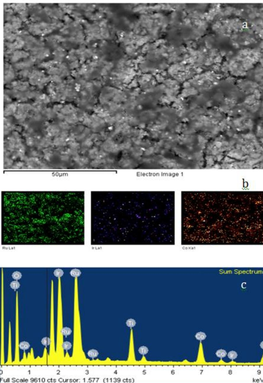
**Figure 2.** (a) SEM micrographs, (b) local mapping analysis, and (c) EDS spectrum of the Ti/RuIrCo(40%:40%:20%)O<sub>x</sub> electrode prepared using conventional thermal decomposition methods.
