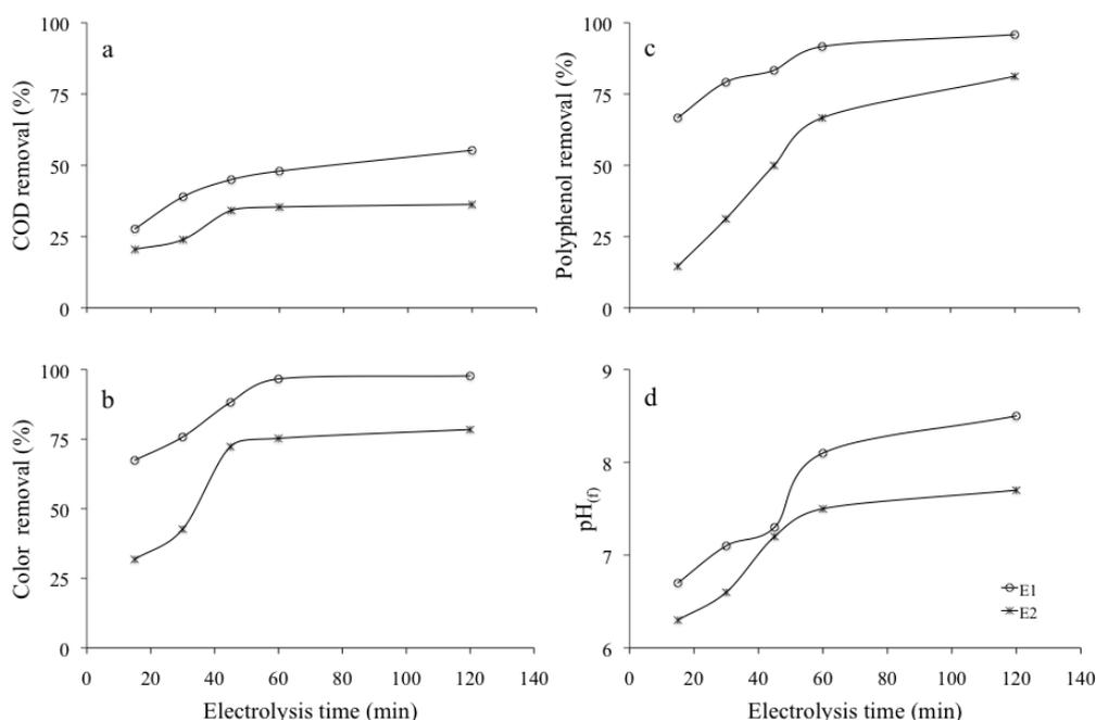
**Figure 3.** Percent removal of (a) COD, (b) color, and (c) polyphenols. (d) pH of the wastewater as a function of the electrolysis time. Anodes: E1 (Ti/RuO<sub>2</sub>) and E2 (Ti/RuIrCo(40%:40%:20%)O<sub>x</sub>). pH (initial) = 6.2, cell potential difference of 6 V, without the addition NaCl.
