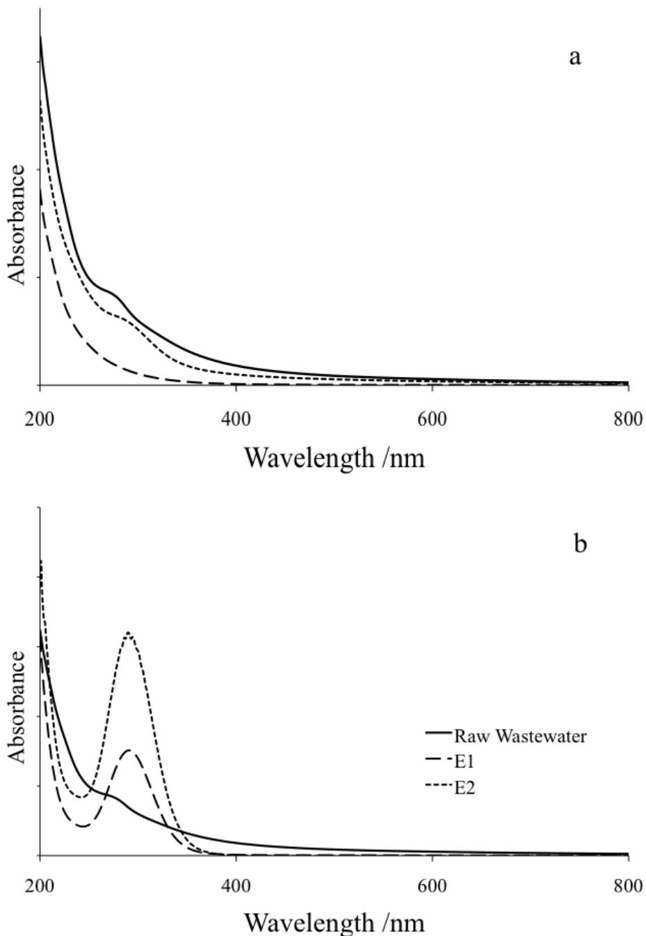
**Figure 5.** UV-Vis spectra of the paper industry wastewater after electrochemical oxidation at the E1 or E2 anodes. Anodes: E1 (Ti/RuO<sub>2</sub>) and E2 (Ti/RuIrCo(40%:40%:20%)O<sub>x</sub>). pH (initial) = 6.2, cell potential difference of 6 V. a) without NaCl, or b) with NaCl (5.0 g/L).
