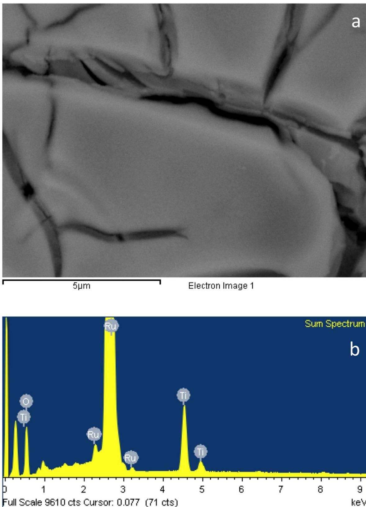
**Figure 1.** (a) SEM micrographs and (b) EDS spectrum of the Ti/RuO<sub>2</sub> electrodes prepared via a conventional thermal decomposition route.
