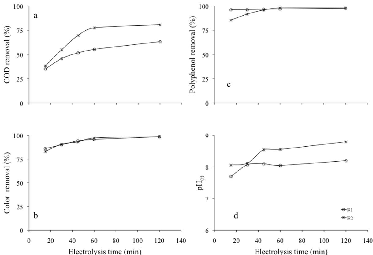
**Figure 4.** Percent removal of (a) COD, (b) color, and (c) polyphenols. (d) pH of the wastewater as a function of the electrolysis time. Anodes: E1 (Ti/RuO<sub>2</sub>) and E2 (Ti/RuIrCo(40%:40%:20%)O<sub>x</sub>). pH (initial) = 6.2, cell potential difference of 6 V, with the electrolyte NaCl (5.0 g/L).
