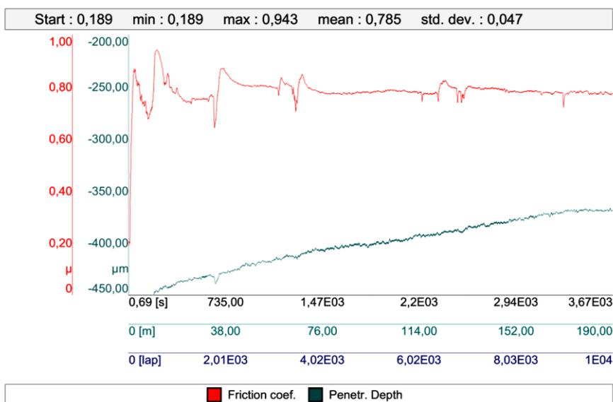
**Figure 2.** The friction coefficient on the surface of Cr<sub>galv</sub> coating and penetration depth of WC ball as a function of conditions of Pin-on-Disc test
