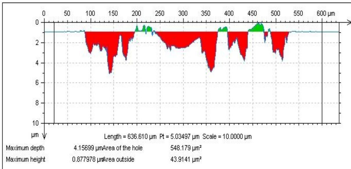
**Figure 3.** Depth of the wear Cr<sub>PVD</sub> coating tested with the WC ball
