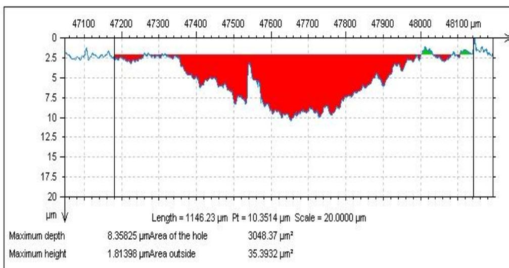
**Figure 4.** Depth of wear of Cr<sub>galv</sub> coating tested with WC ball
