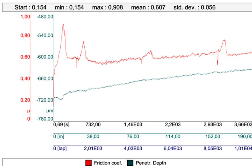
**Figure 1.** The friction coefficient on the surface of Cr<sub>PVD</sub> coating and penetration depth of the WC ball as a function of conditions of Pin-on-Disc test
