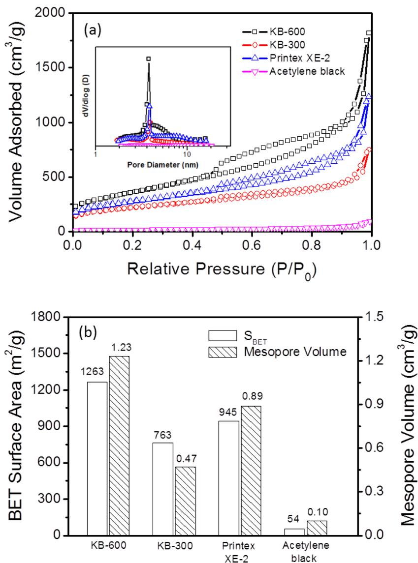
**Figure 1.** (a) Nitrogen adsorption and desorption isotherms of the carbon black samples: the inset shows their pore size distribution. (b) The BET surface area and mesopore volume of the carbon black samples.
