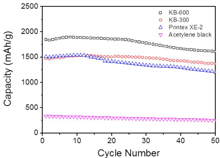
**Figure 3.** Cycle performance of Li/LiAlCl<sub>4</sub>·3SO<sub>2</sub>/SO<sub>2</sub> rechargeable batteries.
