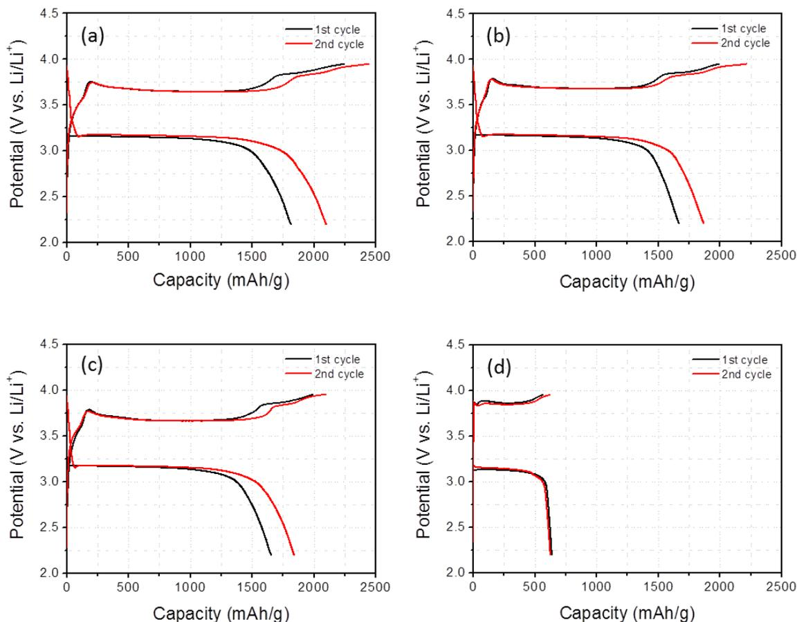
**Figure 2.** Charge/discharge curves for the first two cycles of  $\text{Li}/\text{LiAlCl}_4 \cdot 3\text{SO}_2/\text{SO}_2$  batteries with different carbon black materials: (a) KB-600, (b) KB-300, (c) Printex XE-2, and (d) acetylene black.
