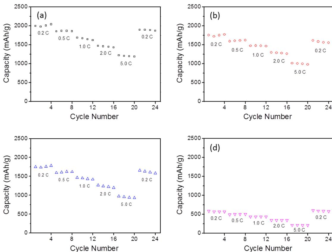
**Figure 4.** Rate properties of Li/LiAlCl<sub>4</sub>·3SO<sub>2</sub>/SO<sub>2</sub> rechargeable batteries: (a) KB-600, (b) KB-300, (c) Printex XE-2, and (d) acetylene black.
