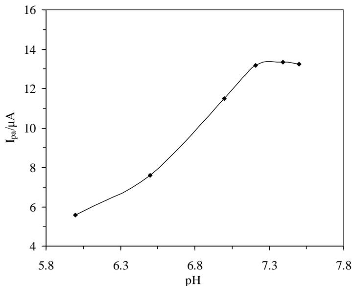
**Figure 4** The influence of pH on the DPV oxidation peak current of matrine.
