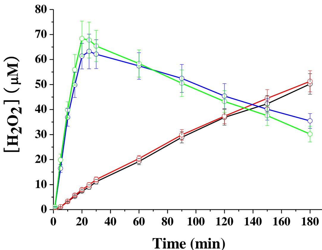
**Figure 4.** Variations of  $[\text{H}_2\text{O}_2]$  generated by free Cu(II) (blue) at pH 7.4 and by mini- $\alpha\text{A}$ -crystallin-Cu(II) at pH 7.4 (black), 6.8 (red) and 6.0 (green). The concentrations of Cu(II) and mini- $\alpha\text{A}$ -crystallin are the same as those in Fig. 2.
