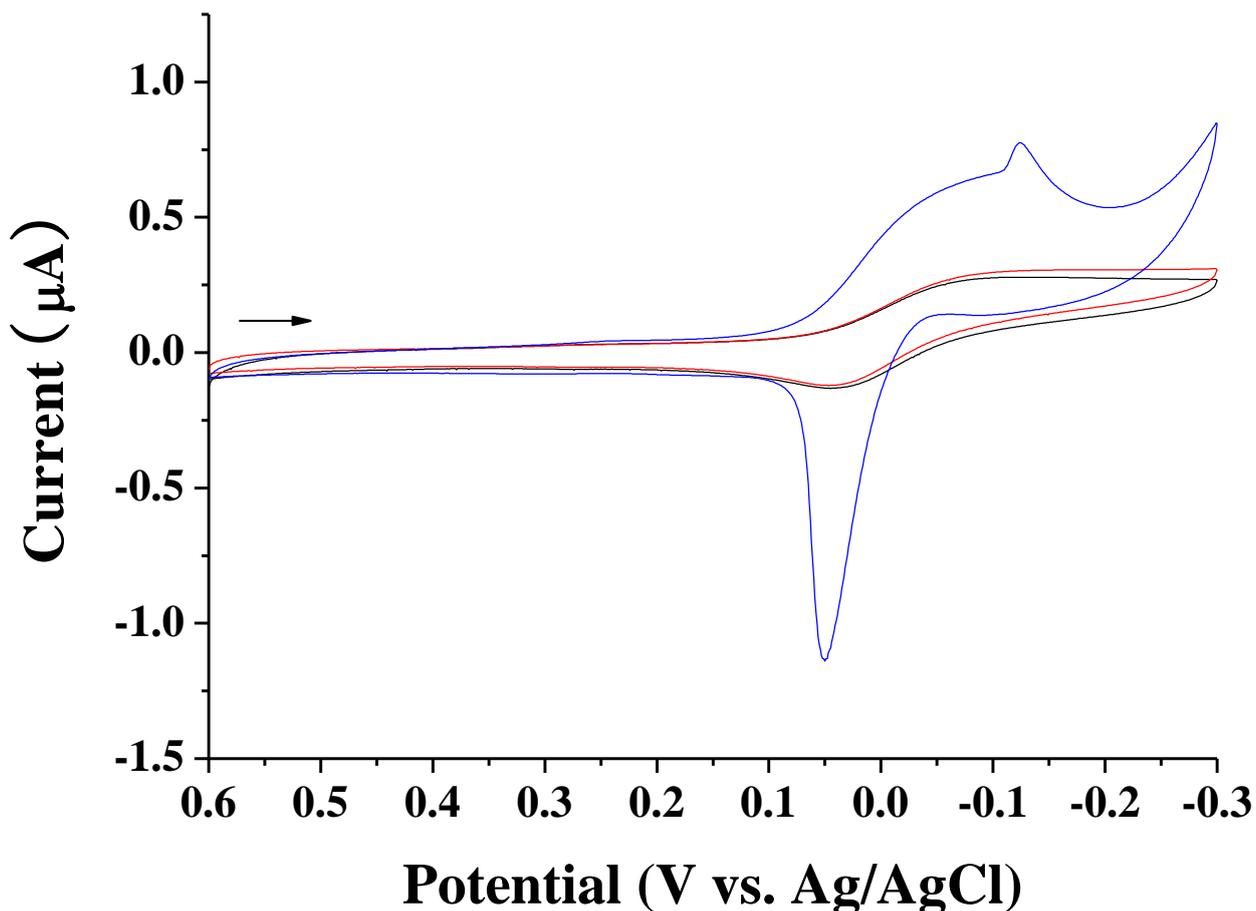
**Figure 3.** CVs of mini- $\alpha$ A-crystallin–Cu(II) at different pH values: 7.4 (black), 6.8 (red) and 6.0 (blue). The other experimental conditions were the same as those in Fig. 1.
