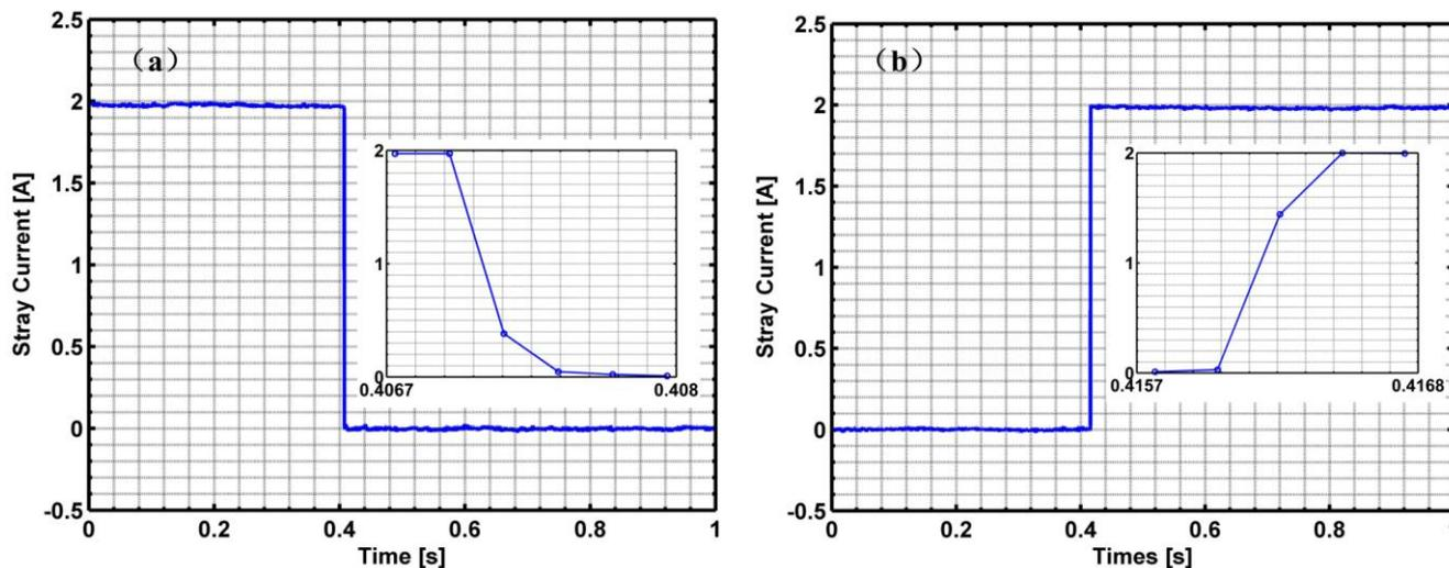
**Figure 5.** Transit response test results: (a) step-down signal; (b) step-up signal.
