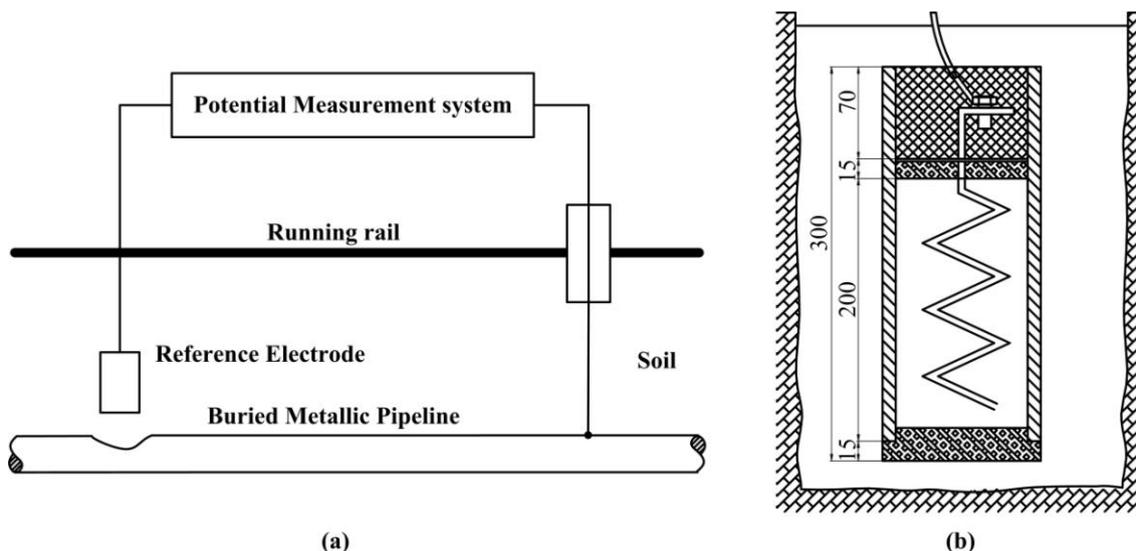
**Figure 1.** Polarization potential measurement method of buried metallic pipeline: (a) measurement system; (b) Cu/CuSO<sub>4</sub> electrode.
