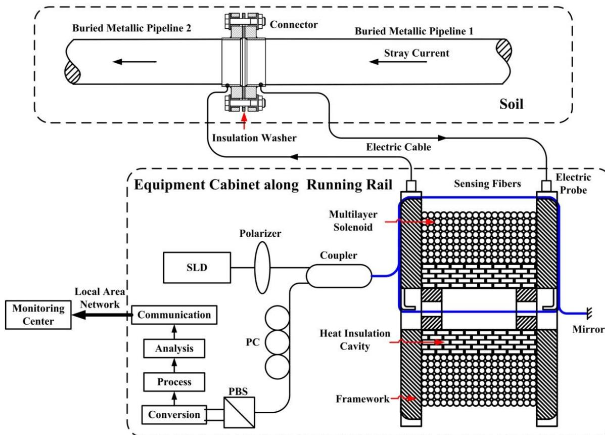
**Figure 2.** An optical fiber sensing system to measure stray current.
