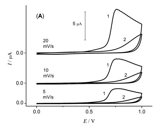
**Figure 3A.** Cyclic voltammograms for the oxidation and polymerisation of using a gold working electrode with a diameter of 1.6 mm at various sweep rates of 0.1 mol  $L^{-1}$  3-aminophenol in 0.1 mol  $L^{-1}$  sulphuric acid. The first two CV's shown at each sweep rate.
