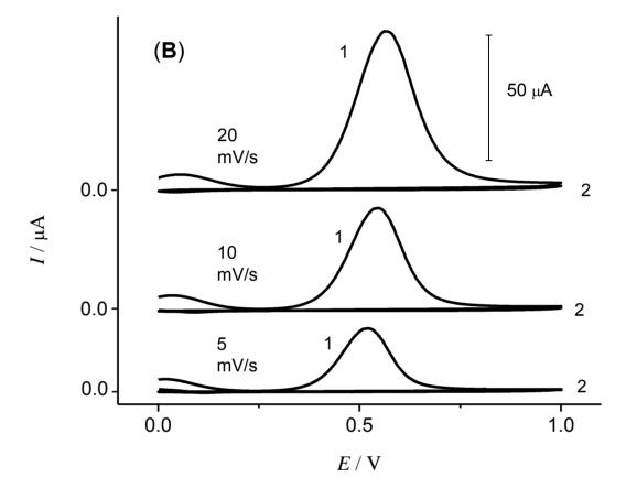
**Figure 4B.** Cyclic voltammograms for the oxidation and polymerisation of using a gold working electrode with a diameter of 1.6 mm at various sweep rates of 0.1 mol  $L^{-1}$  3-aminobenzyl alcohol in 0.1 mol  $L^{-1}$  sodium hydroxide. The first two CV's shown at each sweep rate.
