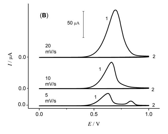
**Figure 1B.** Cyclic voltammograms for the oxidation and polymerisation in neutral, aqueous solutions using a gold working electrode with a diameter of 1.6 mm at various sweep rates of 0.1 mol L<sup>-1</sup> of 3-aminobenzyl alcohol. The first two CV's shown at each sweep rate.
