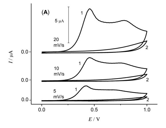
**Figure 1A.** Cyclic voltammograms for the oxidation and polymerisation in neutral, aqueous solutions using a gold working electrode with a diameter of 1.6 mm at various sweep rates of 0.1 mol L<sup>-1</sup> of 3-aminophenol. The first two CV's shown at each sweep rate.
