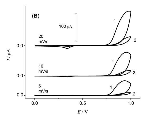
**Figure 3B.** Cyclic voltammograms for the oxidation and polymerisation of using a gold working electrode with a diameter of 1.6 mm at various sweep rates of 0.1 mol  $L^{-1}$  3-aminobenzyl alcohol in 0.1 mol  $L^{-1}$  sulphuric acid. The first two CV's shown at each sweep rate.
