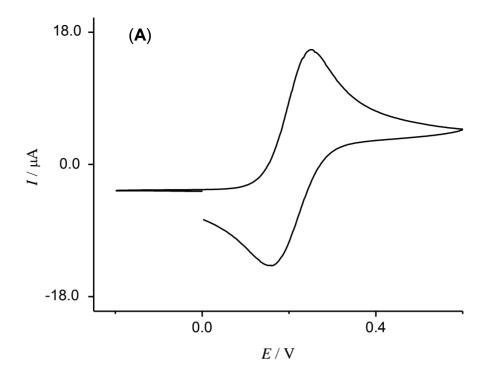
**Figure 5A.** A typical cyclic voltammogram run of polished gold electrode tested in 5.0 mmol L<sup>-1</sup> ferri/ferro cyanide 0.1 mol L<sup>-1</sup> KCl solution (before polymerisation).
