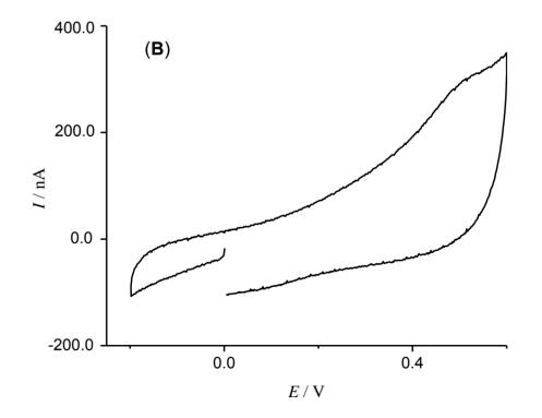
**Figure 5B.** A typical cyclic voltammogram run of the same gold electrode after the polymerisation of 3-aminobenzyl alcohol in  $0.1 \text{ mol } L^{-1}$  sodium hydroxide.
