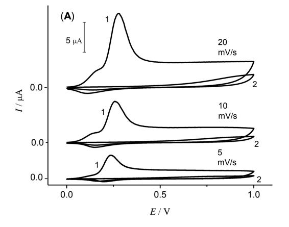
**Figure 4A.** Cyclic voltammograms for the oxidation and polymerisation of using a gold working electrode with a diameter of 1.6 mm at various sweep rates of 0.1 mol  $L^{-1}$  3-aminophenol in 0.1 mol  $L^{-1}$  sodium hydroxide. The first two CV's shown at each sweep rate.
