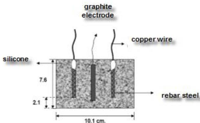
**Figure 1.** Test system for electrochemical techniques
