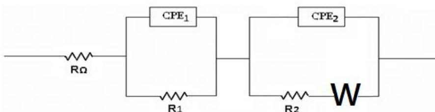
**Figure 6.** Circuit used for fitting, the electrochemical behavior of zinc coated steel and embedded in concrete alternative.
