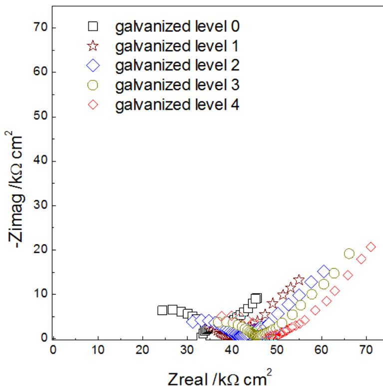
**Figure 5.** Nyquist plot corresponding to systems where the steel is covered with zinc; and embedded in the alkali-activated slag concrete. With increasing level of assessment, electrochemical parameters generate greater protection
