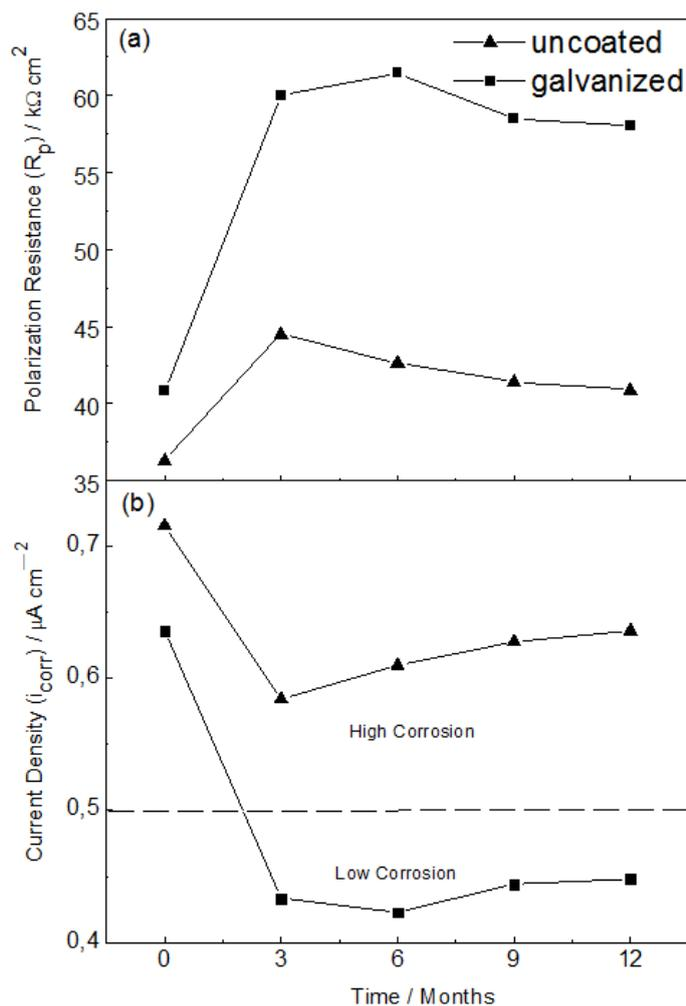
**Figure 2.** Rp variation for different systems by LPR technique.
