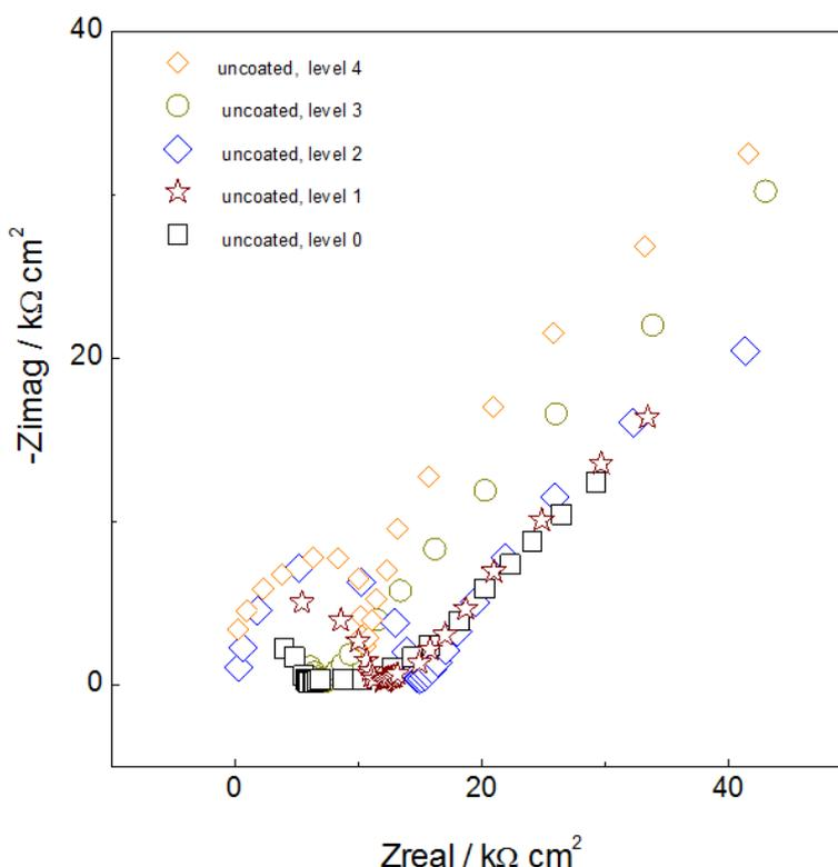
**Figure 3.** Nyquist plot that assesses the evolution of the electrochemical behavior of uncoated steel; embedded in the concrete of alkali activation.
