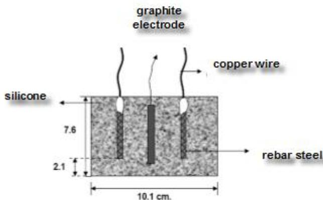
**Figure 1.** Test system for electrochemical techniques
