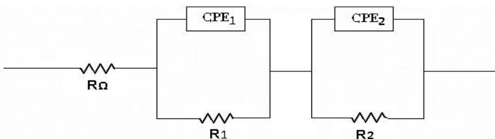
**Figure 4.** Equivalent circuit representing the behavior of uncoated steel embedded in concrete alkali activated slag with exposure to chloride.
