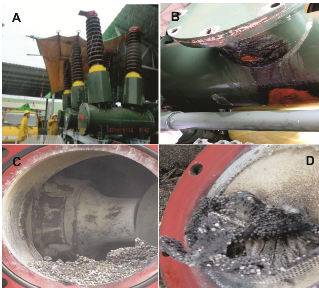
Figure 1. The \text{SF}_6 reactor tank (A), closed (B) and opened pole tank (C) with molecular sieves and lit of the pole tank (D).
