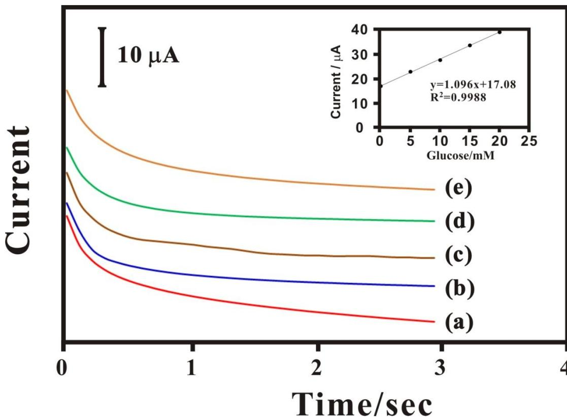
**Figure 5.** Amperometric *i-t* response obtained at Nafion/Pd-GOx modified SPCE in the absence (a) and presence of Human blood (b) and each addition of 0.005 M glucose (c–e). Working potential = 0.4 V.
