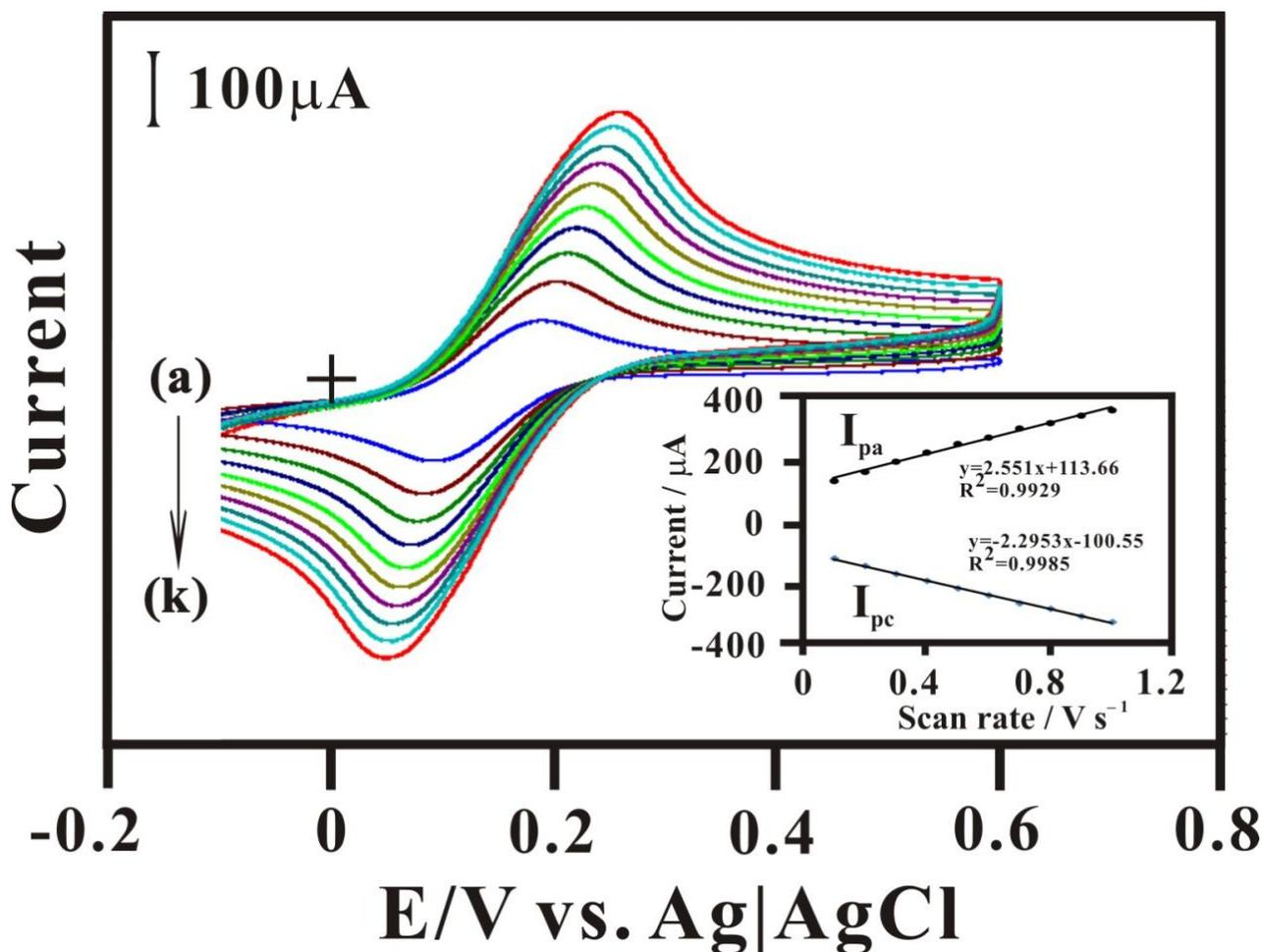
**Figure 2.** The cyclic voltammetry response of Nafion/Pd-GOx modified SPCE in pH 7 at sweeping of different scans rate from 0.01 to 0.1 V/s. Inset shows the calibration plot for scan rate vs. current response.
