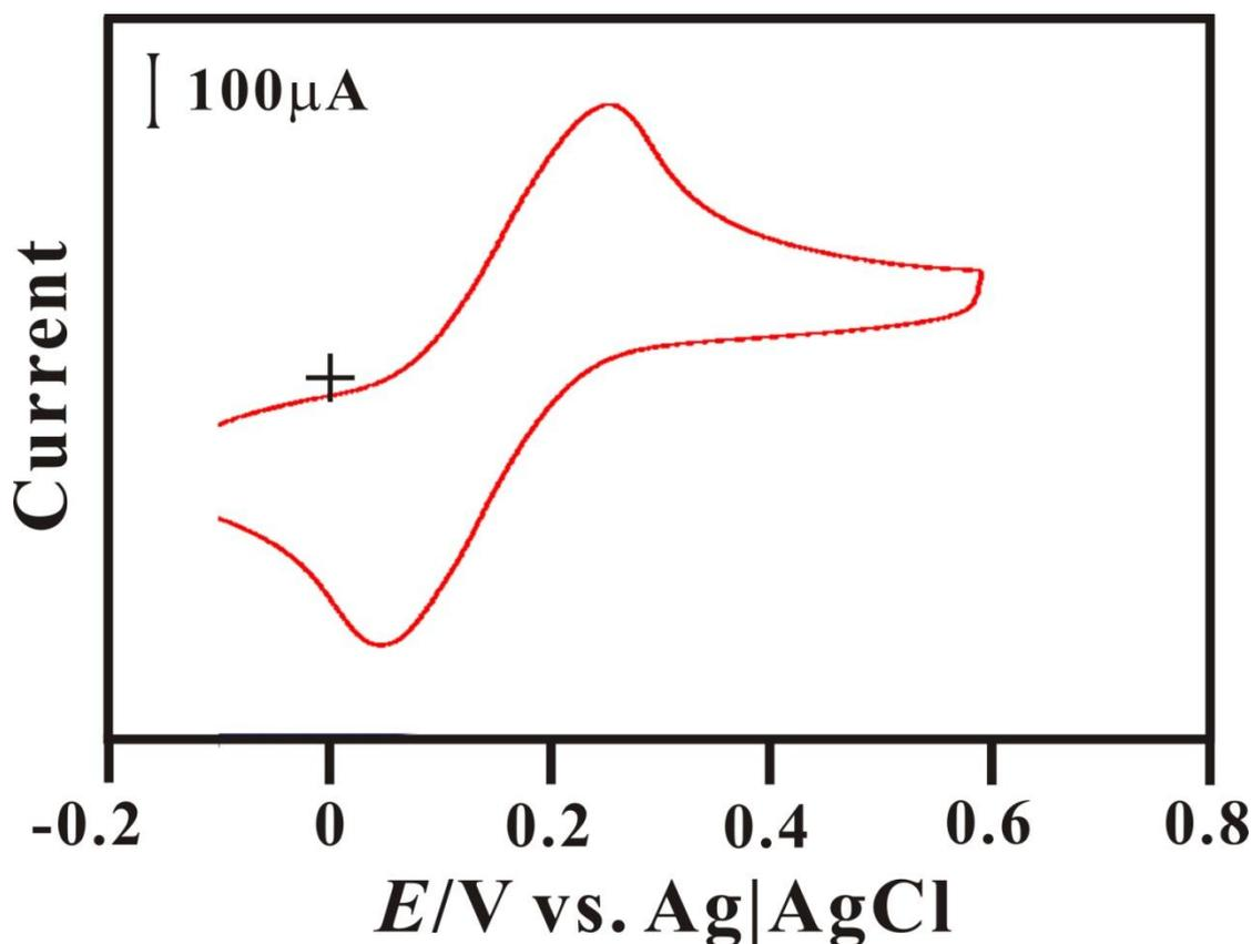
**Figure 1.** Cyclic voltammery response of a Nafion/Pd-GOx modified SPCE in pH 7 containing 1 mM  $\text{K}_4\text{Fe}(\text{CN})_6$  at a scan rate of 0.1 V/s.
