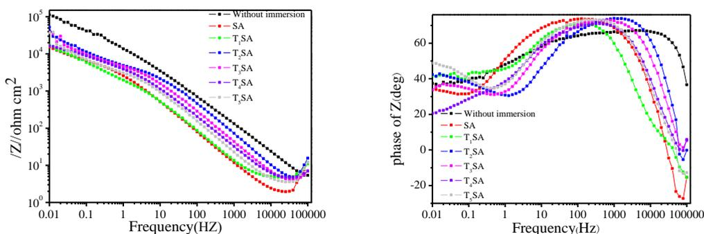
**Figure 5.** Impedance response (a) and phase shift (b) of anodic film immersed in sulfuric acid (SA) and sulfuric acid with 10g/L tartaric acid (T<sub>1</sub>SA), 30g/L tartaric acid (T<sub>2</sub>SA), 50g/L tartaric acid (T<sub>3</sub>SA), 70g/L tartaric acid (T<sub>4</sub>SA), 90g/L tartaric acid (T<sub>5</sub>SA).
