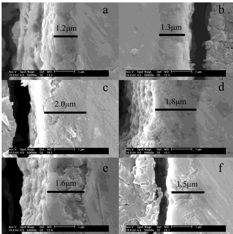
**Figure 2.** SEM images of titanium alloy anodised in sulfuric acid without tartaric acid (a) and with 10g/L tartaric acid (b), 30g/L tartaric acid (c), 50g/L tartaric acid (d), 70g/L tartaric acid (e) and 90g/L tartaric acid (f).
