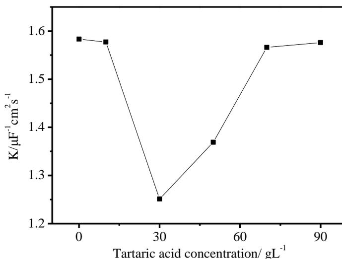
**Figure 7.** Dissolution rate of anodic film immersed in sulfuric acid and sulfuric acid with different tartaric acid additions.
