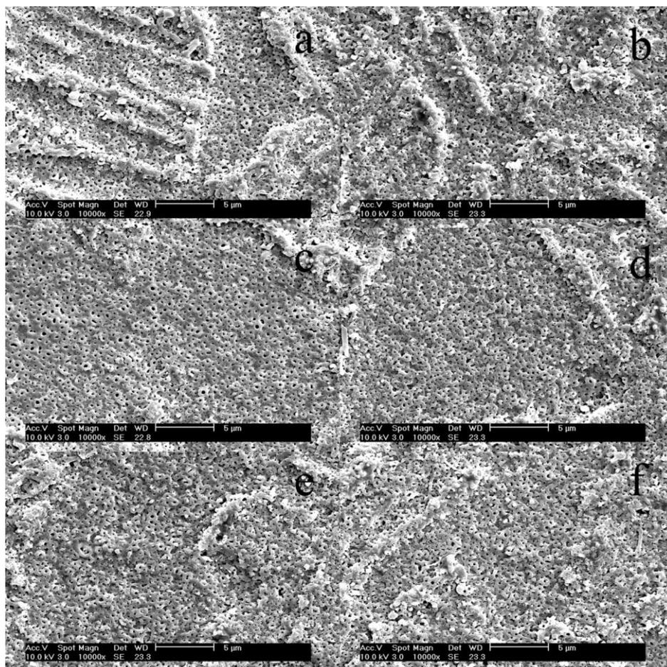
**Figure 1.** SEM images of titanium alloy anodised in sulfuric acid without tartaric acid (a) and with 10g/L tartaric acid (b), 30g/L tartaric acid (c), 50g/L tartaric acid (d), 70g/L tartaric acid (e) and 90g/L tartaric acid (f).
