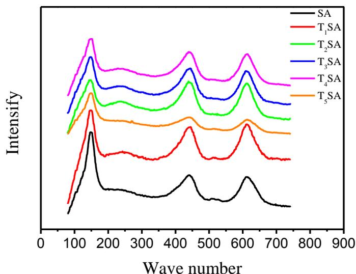
**Figure 3.** Raman spectra of anodic films formed in sulfuric acid without tartaric acid (SA) and sulfuric acid with 10g/L (T<sub>1</sub>SA), 30g/L (T<sub>2</sub>SA), 50g/L (T<sub>3</sub>SA), 70g/L (T<sub>4</sub>SA) and 90g/L (T<sub>5</sub>SA) tartaric acid.
