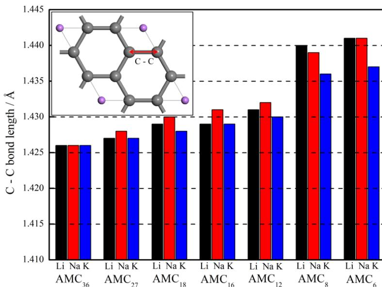
**Figure 5.** The C-C bond lengths of carbon six-membered ring in the carbon layer intercalated with alkali metal ions
