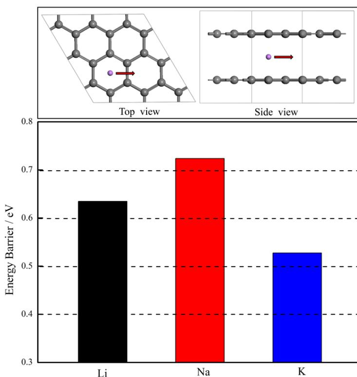
**Figure 6.** The energy barriers of the alkali metal ion jumps between the sites in the graphite
