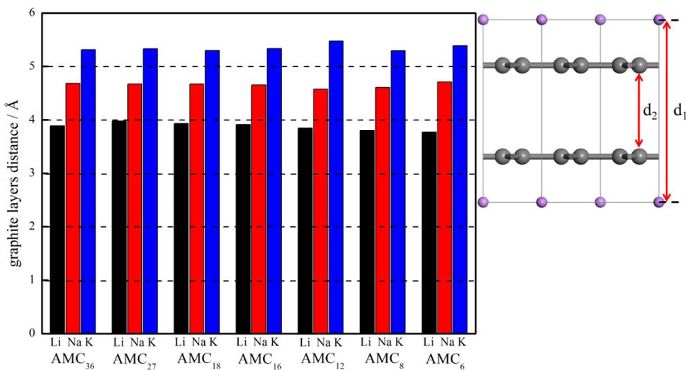
**Figure 4.** The distances between the carbon layers intercalated with alkali metal ions
