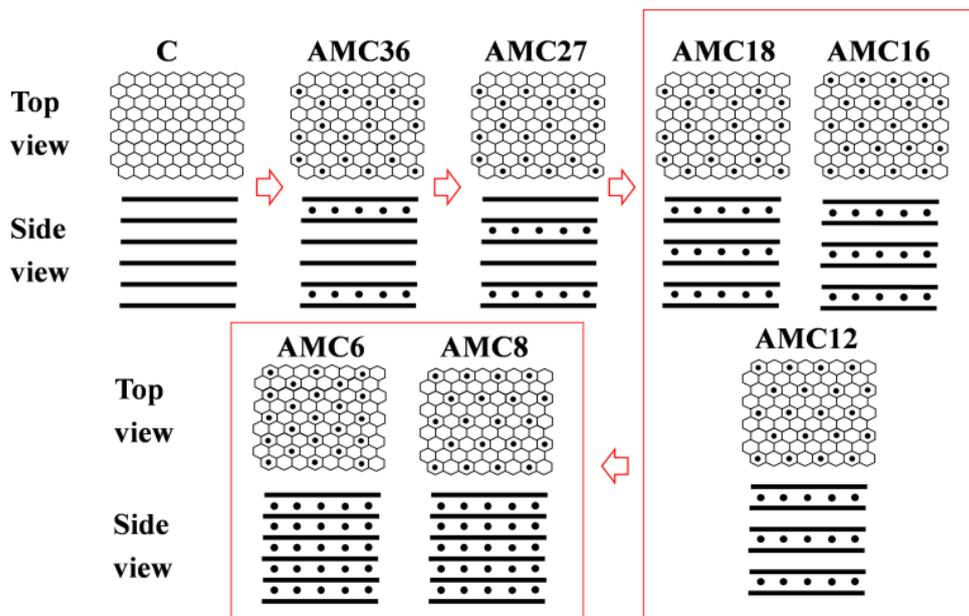
Figure 1. Staged structures of AM-GICs
