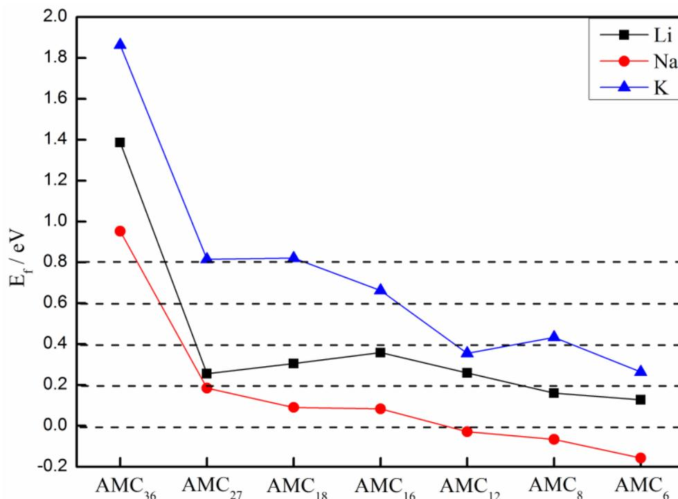
**Figure 3.** The formation energies of AM-GICs with different intercalated density of alkali metal
