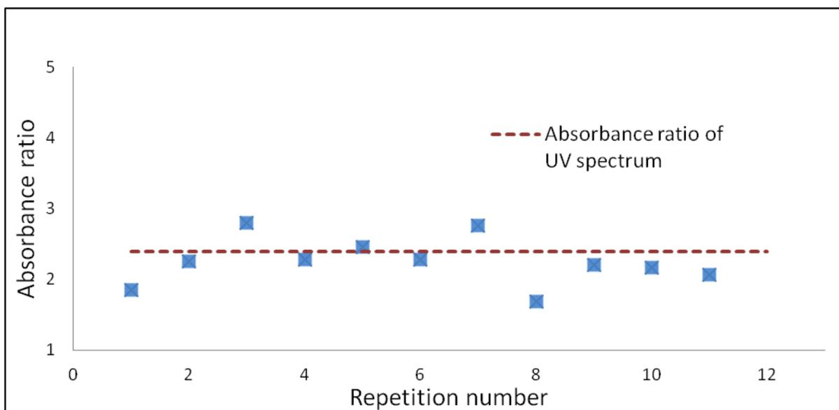
**Figure 3.** Calculated absorbance ratios of the glucose peak during repeated analyses of a selected concentration of reference solution (60 ppm). The dashed line represents the calculated value of absorbance ratio from the UV spectrum in Fig. 2.
