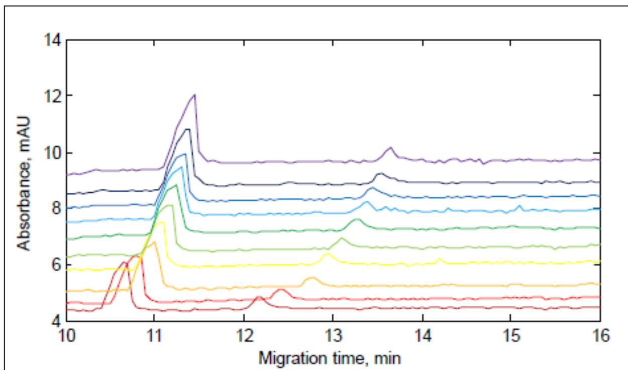
**Figure 4.** Examples of 10 electropherograms of sequential analytical runs. Peaks in the figure are system peak and sucrose.
