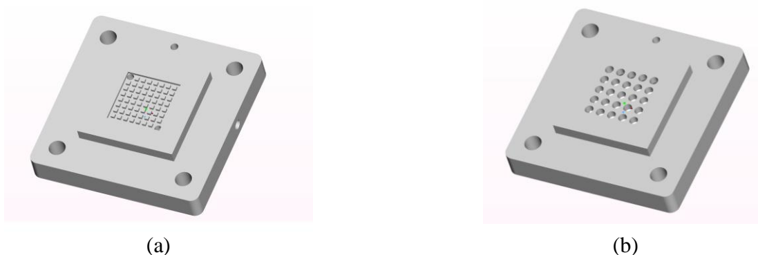
Figure 1. The configurations of anode (a) and cathode (b) plates of the air-breathing DMFC.
