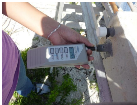
Figure 3. Measuring concrete internal RH and T.
