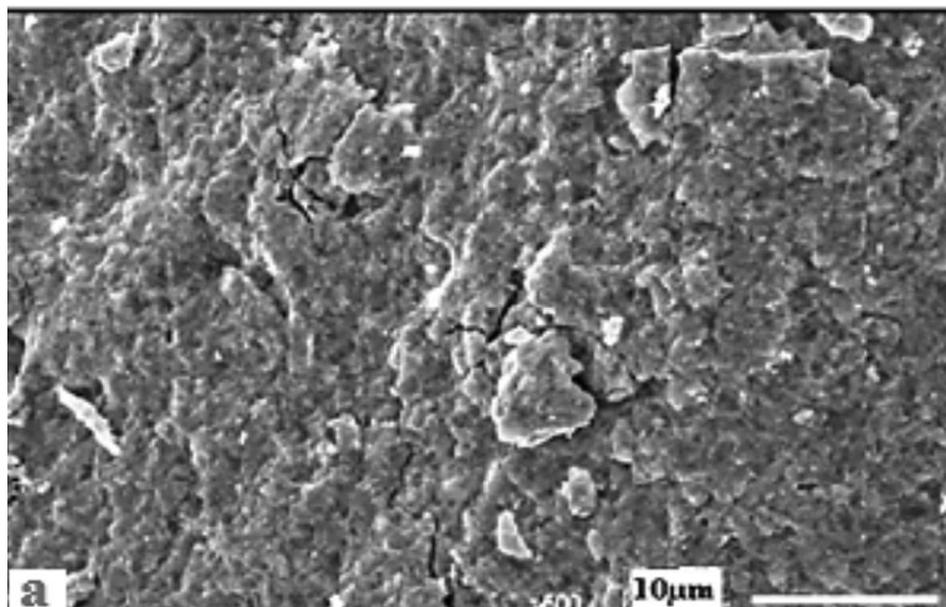
**Figure S2.** SEM of PSTM nanocomposite cation-exchange material [Ref. 41, with permission].
