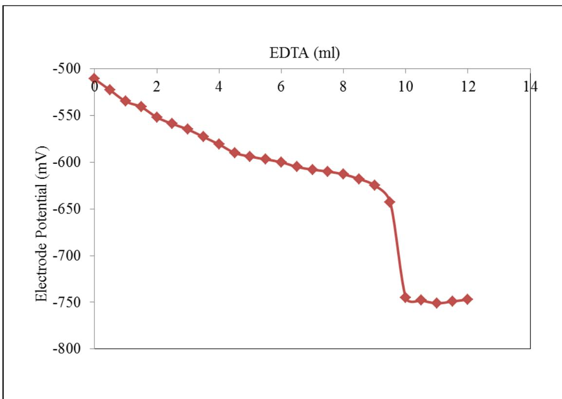
**Figure 7.** Potentiometric titration curve of solution of  $\text{Pb}(\text{II})$  ions against EDTA solution.
