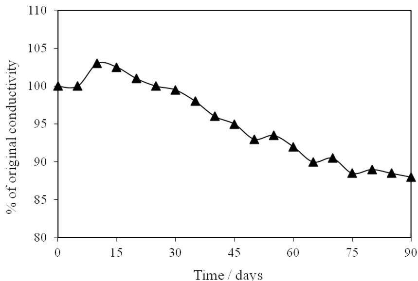
**Figure 5.** Conductivity versus time of exposure to laboratory air for polyaniline Sn(IV) tungstomolybdate composite material (HCl treated).
