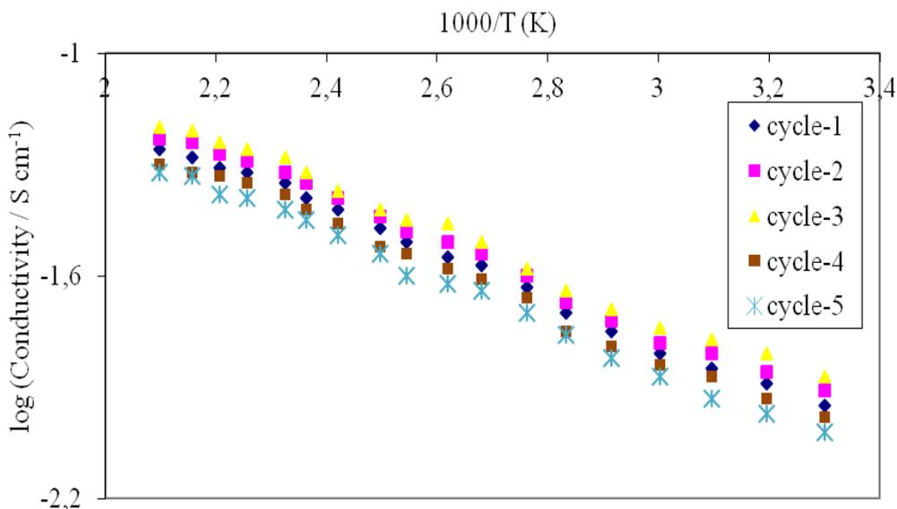
**Figure 4.** Arrhenius plots of retention of dc electrical conductivity for polyaniline Sn(IV) phosphate (HCl treated) during heating cooling cycles up to 200 °C.
