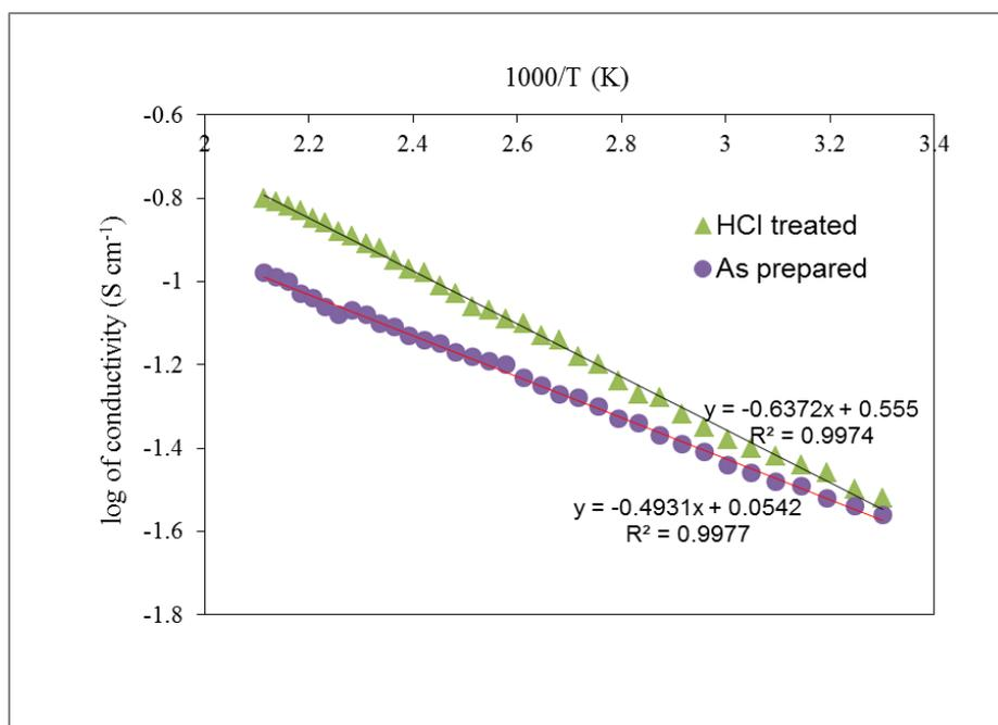
**Figure 2.** Arrhenius plots for polyaniline Sn(IV) tungstomolybdate composite material (as prepared and HCl treated).
