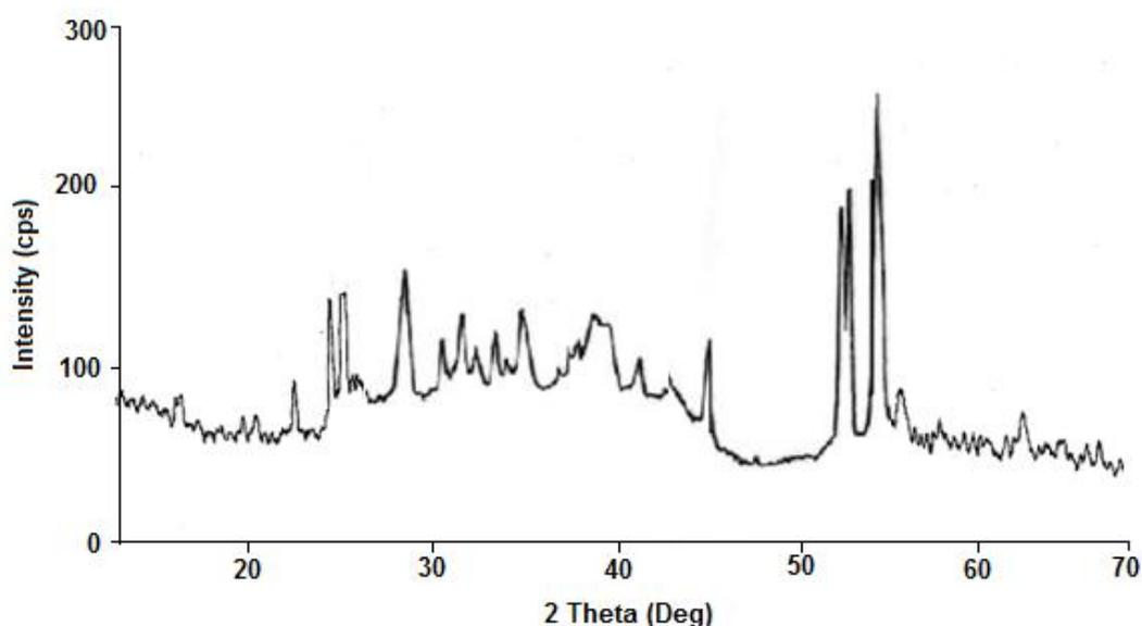
**Figure 1.** XRD of PSTM nanocomposite cation-exchange material.
