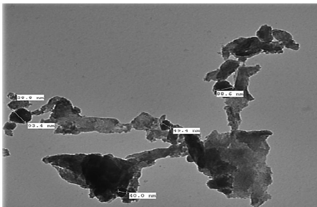
**Figure S3.** TEM of PSTM nanocomposite cation-exchange material [Ref. 41, with permission].
