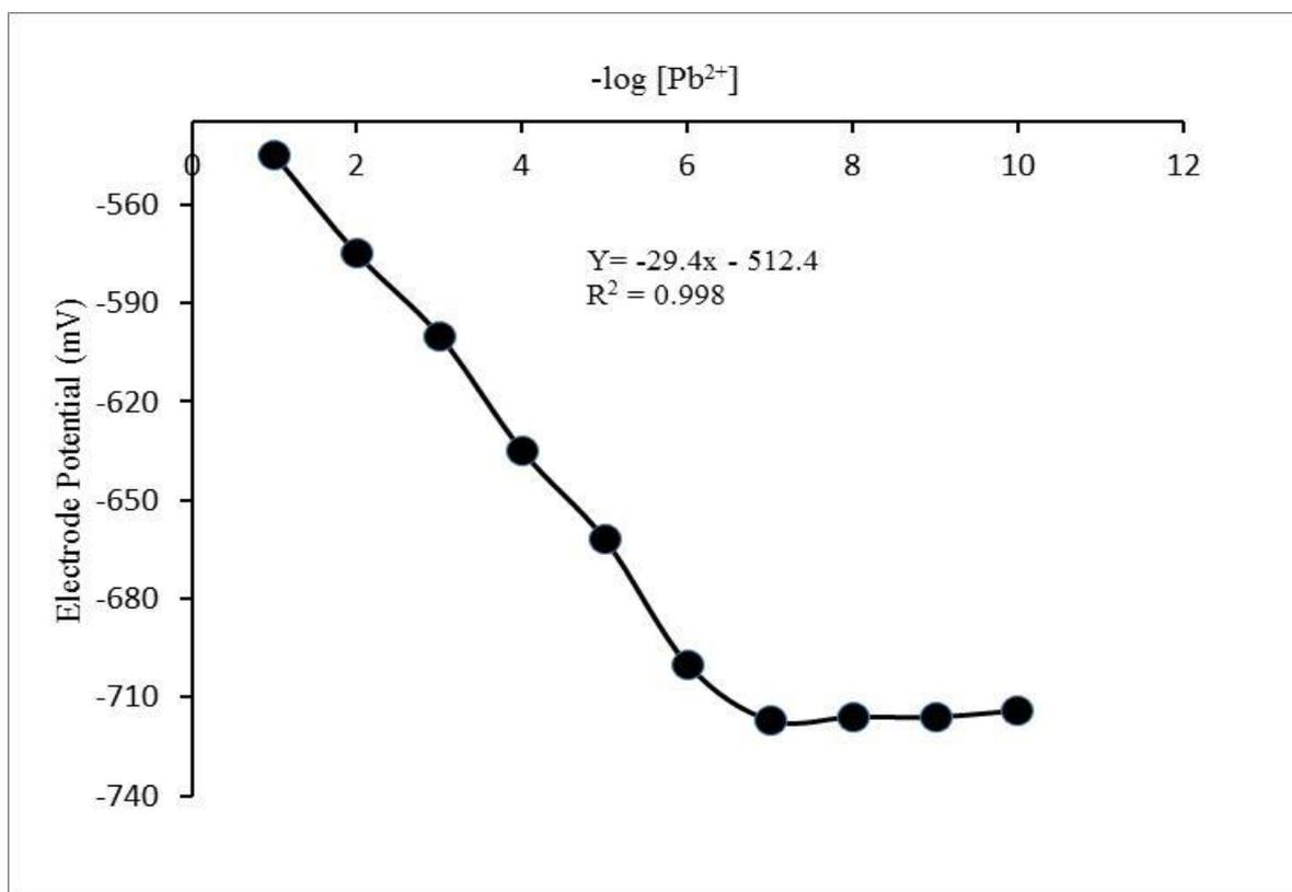
**Figure 6.** Calibration graph of Pb(II) ion-selective PSTM membrane electrode.
