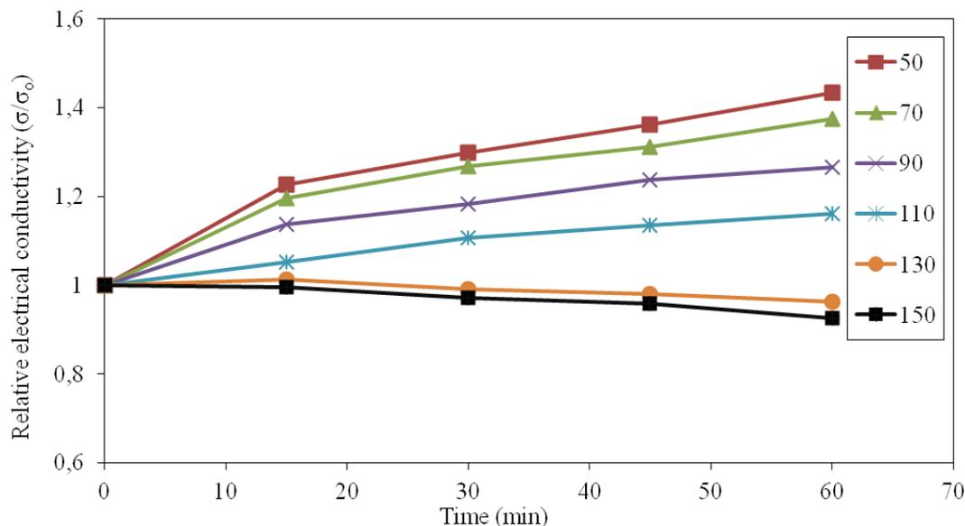
**Figure 3.** Isothermal stability of polyaniline Sn(IV) tungstomolybdate composite material (HCl treated) in terms of retention of DC electrical conductivity with respect to time at 50, 70, 90, 110, 130 and 150 °C.
