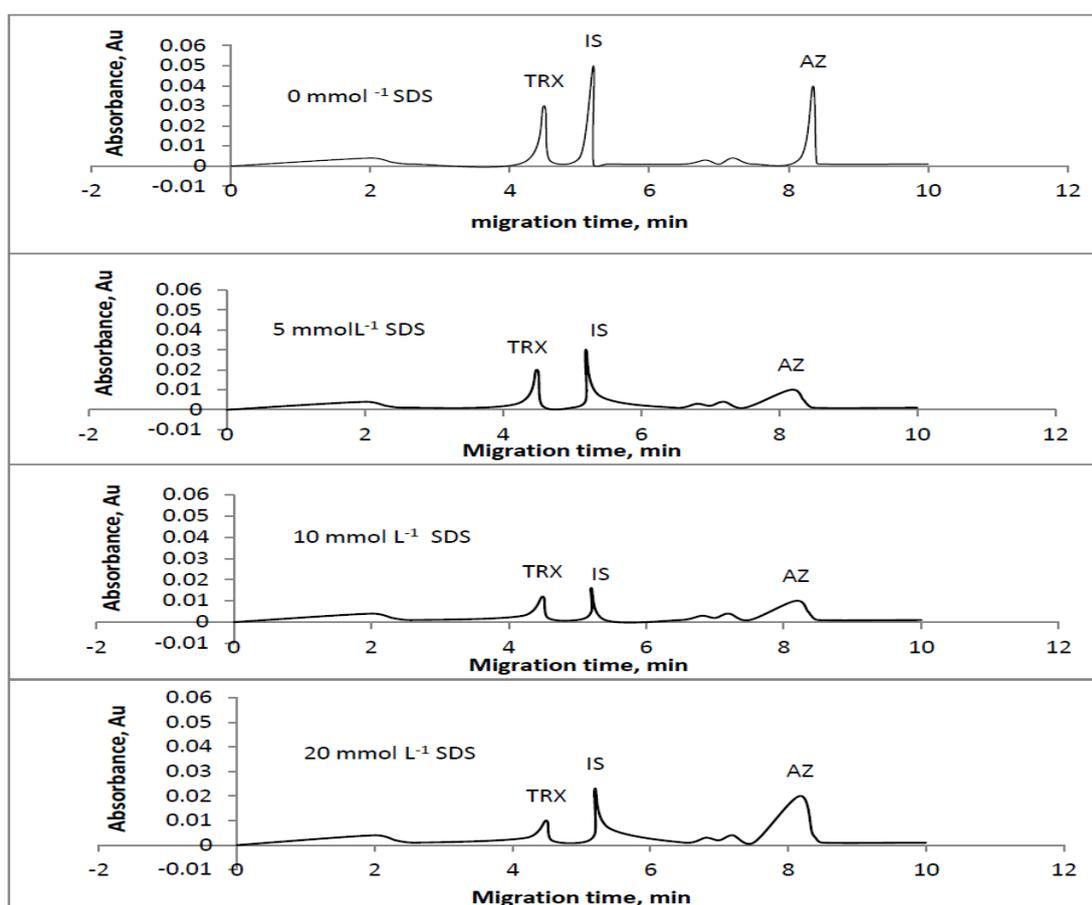
**Figure 4.** Effect of SDS (5-20 mmol L<sup>-1</sup>) on separation of TRX; (IS) and AZ; Running buffer; 25 mmol L<sup>-1</sup> sodium tetraborate decahydrate and methanol 80:20% (v/v); injection 90 mbar for 8 s; separation voltage 25 kV; capillary temperature 30°C, DAD detection at 260 nm
