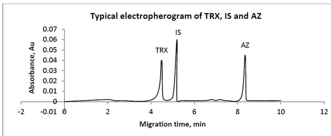
**Figure 6.** Typical electropherogram corresponding to the separation of 100  $\mu\text{g mL}^{-1}$  TRX; 200  $\mu\text{g mL}^{-1}$  IS and 70  $\mu\text{g mL}^{-1}$  AZ
