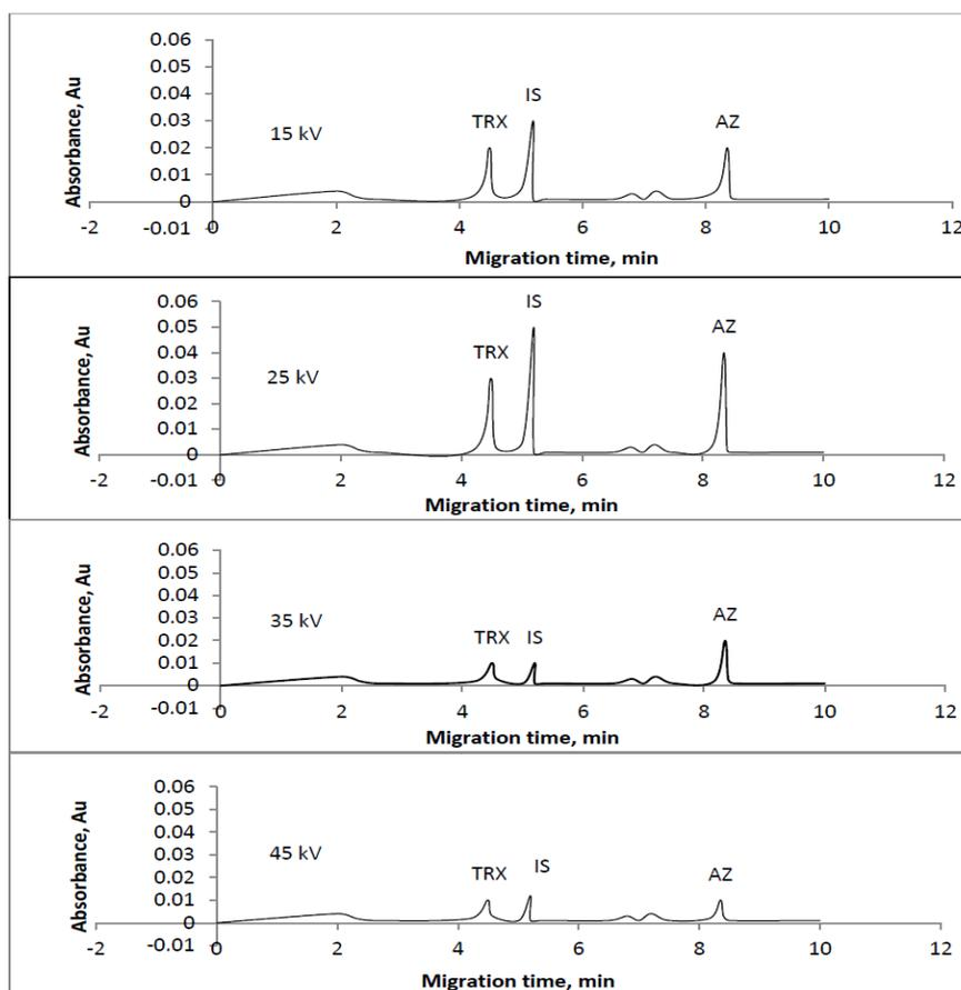
**Figure 5.** Effect of different voltage on separation of TRX; (IS) and AZ; Running buffer; 25 mmol L<sup>-1</sup> sodium tetraborate decahydrate and methanol 80:20% (v/v); injection 90 mbar for 8 s; separation voltage (15-45 kV); capillary temperature 30 °C, DAD detection at 260 nm
