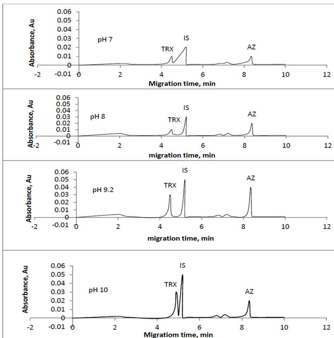
**Figure 3.** Effect of pH value on separation TRX; (IS) and AZ; Running buffer; 25 mmol L<sup>-1</sup> sodium tetraborate decahydrate and methanol 80:20% (v/v); injection 90 mbar for 8 s; separation voltage 25 kV; capillary temperature 30 °C, DAD detection at 260 nm
