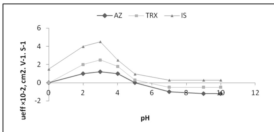
**Figure 2.** Effective mobility curve in function of the pH for TRX, AZ and IS
