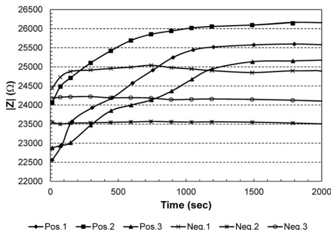
**Figure 5.** Time dependence of the measured impedance during RCA for three positive samples and three negative controls at 472 kHz.
