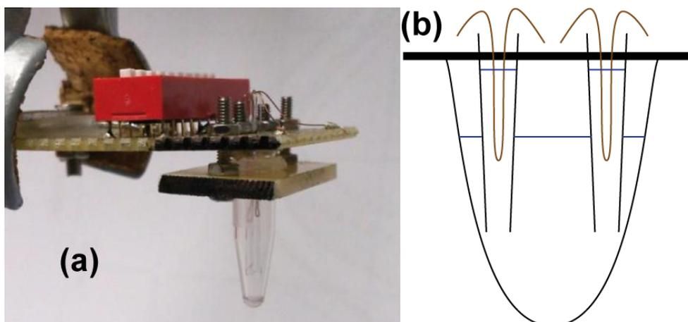
**Figure 2.** (a) Photo and (b) schematic representation of the sensor.
