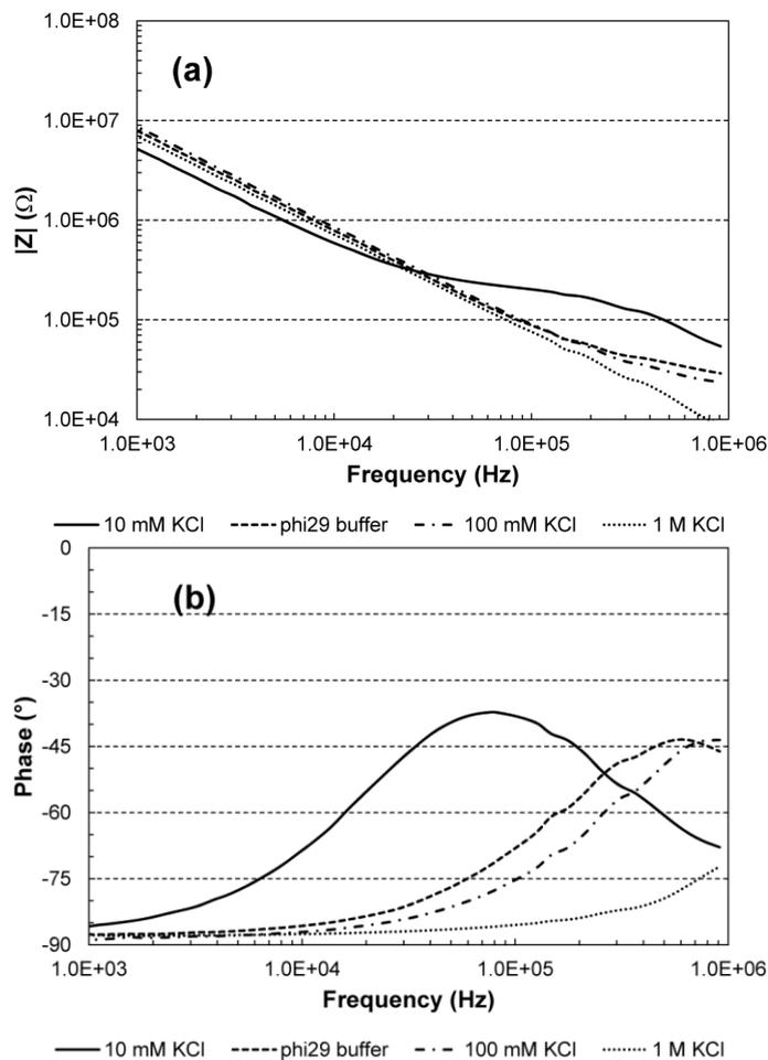
**Figure 3.** Measured impedance spectra for analytes with different electrical conductivities. (a) Absolute value of the impedance, (b) phase angle.
