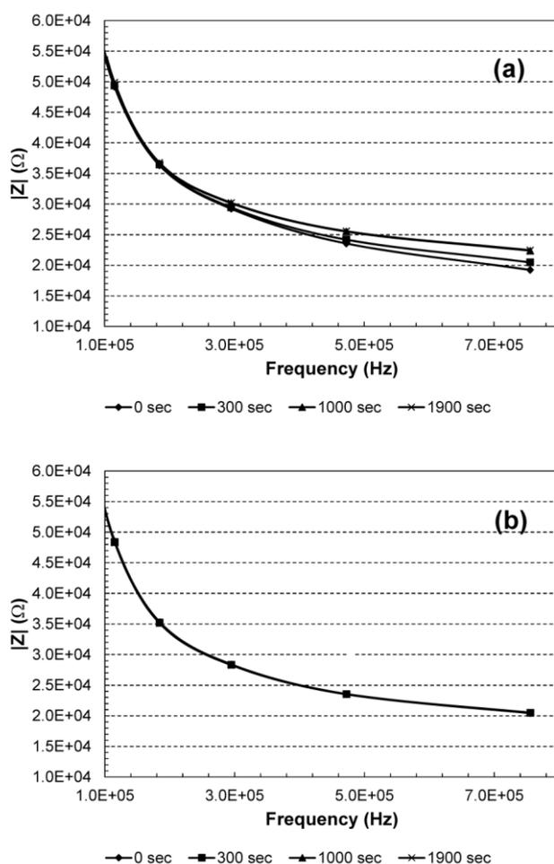
**Figure 4.** Impedance spectra measured at different reaction times for positive samples (a) and negative controls (b).
