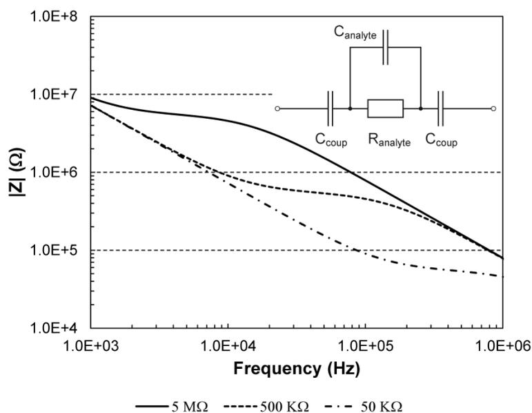
**Figure 1.** Calculated impedance spectra of a C<sup>4</sup> sensor. Values for  $C_{coup}$  and  $C_{analyte}$  are close to those found experimentally in our sensor (44 pF and 2.2 pF, respectively). Spectra were calculated using Matlab.
