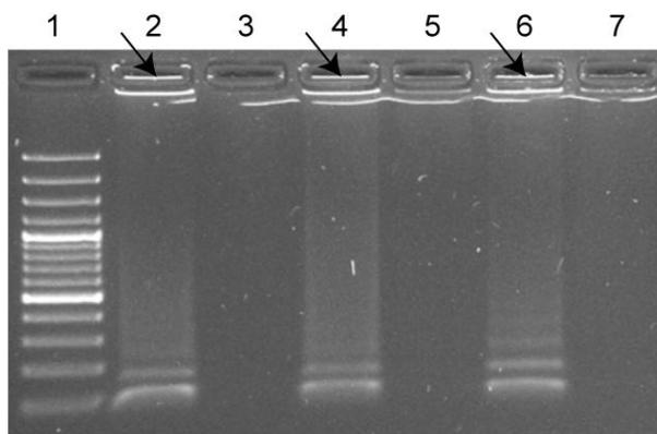
**Figure 6.** Image of agarose gel-electrophoresis; 1:100 bp DNA-Ladder, upper bright bar: 1000 bp, lower bright bar: 500 bp. 2, 4, 6: Positive samples; 3, 5, 7: Negative controls. Amplification products only occurred in positive samples. Long single-strand DNA can not enter the gel and remains in the pocket (indicated by arrows). Shorter single-strand DNA fragments of various lengths were created in the digestion step and appear as multiple bands.
