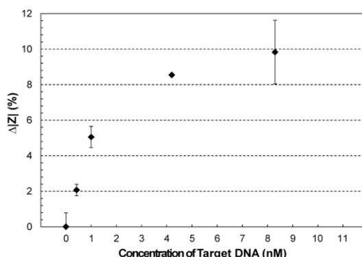
**Figure 7.** Impedance change after 45 minutes amplification time for different DNA target concentrations. The measurement frequency was 472 kHz. The error bars indicate the standard deviation of at least 3 different measurements, except for the point at 4.2 nM, which is a single measurement.
