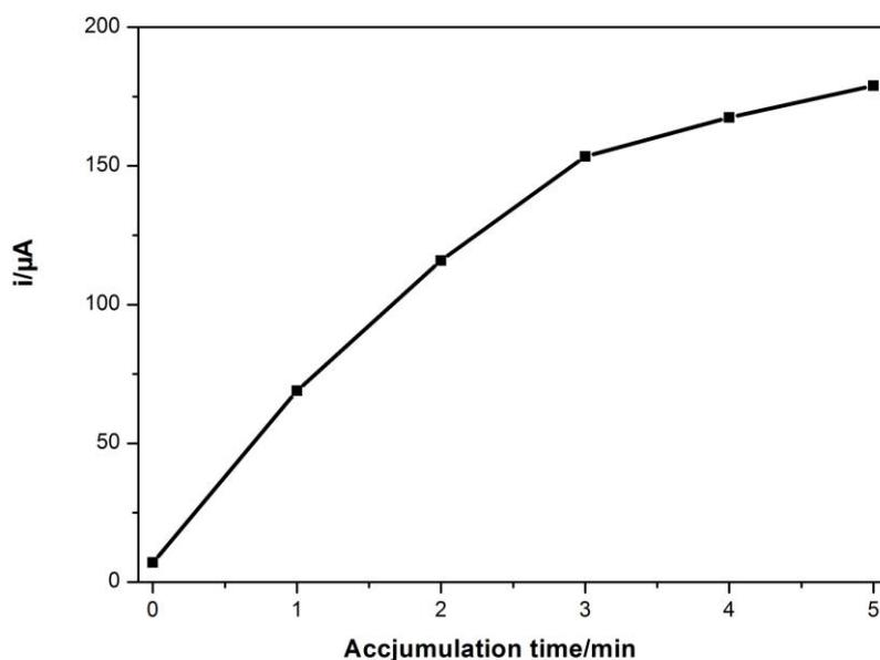
**Figure 6.** The effect of accumulation time on the peak current of  $1 \times 10^{-5} \text{ mol L}^{-1}$  rutin.
