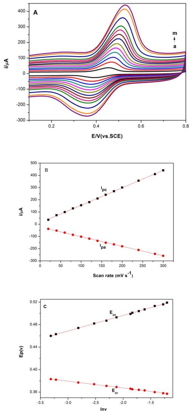
**Figure 5.** (A) Effect of different scan rate (a-k: 20, 40, 60, 80, 100, 120, 140, 160, 180, 200, 240, 280, 300) on the redox behavior of  $1.0 \times 10^{-5} \text{ mol L}^{-1}$  rutin in  $0.2 \text{ mol L}^{-1}$  PBS (pH 3.5) at CCB-GR/GCE. (B) Effect of scan rate on peak current. (C) Effect of scan rate on peak current peak voltage.
