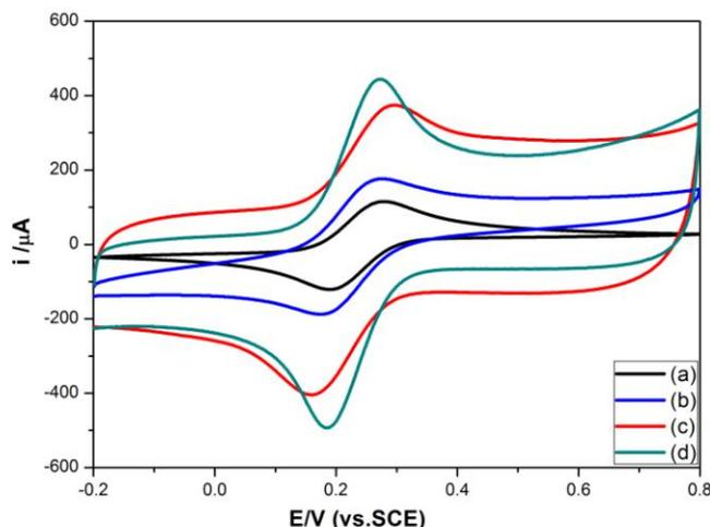
**Figure 2.** Cyclic voltammograms of the bare GCE (a), CCB/GCE (b), GR/GCE (c), CCB-GR/GCE (d), in  $5.0 \text{ mmol L}^{-1} [\text{Fe}(\text{CN})_6]^{3-/4-}$  containing  $0.5 \text{ mol L}^{-1} \text{ KCl}$  solution at the scan rate of  $100 \text{ mV s}^{-1}$ .
