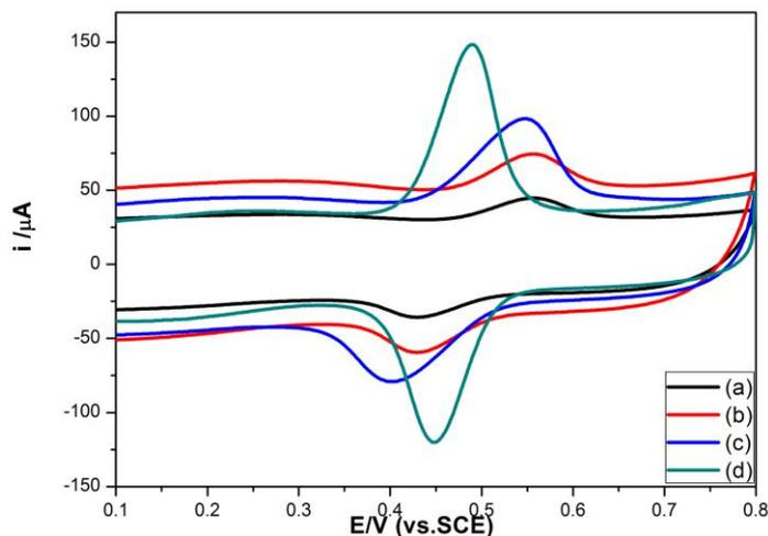
**Figure 3.** Cyclic voltammograms of  $1 \times 10^{-5} \text{ mol L}^{-1}$  rutin at the bare GCE (a), CCB/GCE (b), GR/GCE (c), CCB-GR/GCE (d), in  $0.2 \text{ mol L}^{-1}$  PBS (pH 3.5) at scan rate of  $100 \text{ mV s}^{-1}$ .
