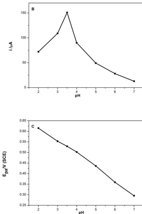
**Figure 4.** (A) Cyclic voltammograms of  $1.0 \times 10^{-5}$  mol L<sup>-1</sup> rutin at CCB-GR/GCE with different pH (a-g: 7.0, 6.0, 5.0, 4.0, 3.5, 3.0, 2.0) at scan rate of 100 mV s<sup>-1</sup>. (B) Effect of pH value on anodic peak currents. (C) Effect of pH value on anodic peak potentials.
