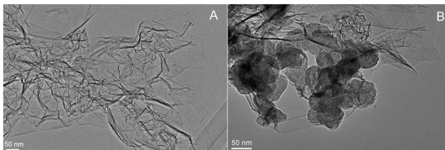
**Figure 1.** TEM images of (A) GR and (B) CCB/GR composite
