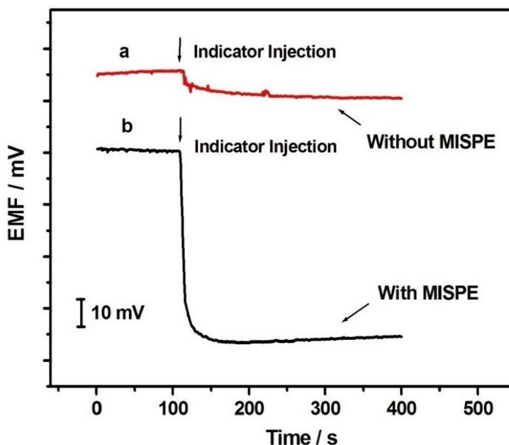
**Figure 5.** Potential responses of the detection system without (a) and with (b) the MISPE cartridge. Concentration of indicator ion,  $3 \times 10^{-5}$  M; sample, 0.5 M NaCl and 10 mg/L fluvic acid. Other conditions as in Figure 2.
