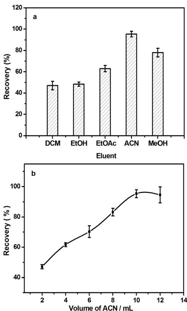
**Figure 3.** Effects of eluent (a), the eluting volume (b), and the eluting flow rate (c) on the recovery of CPF. Each data point represents a mean value  $\pm$  relative standard deviation for three measurements. Other conditions as in Figure 2.
