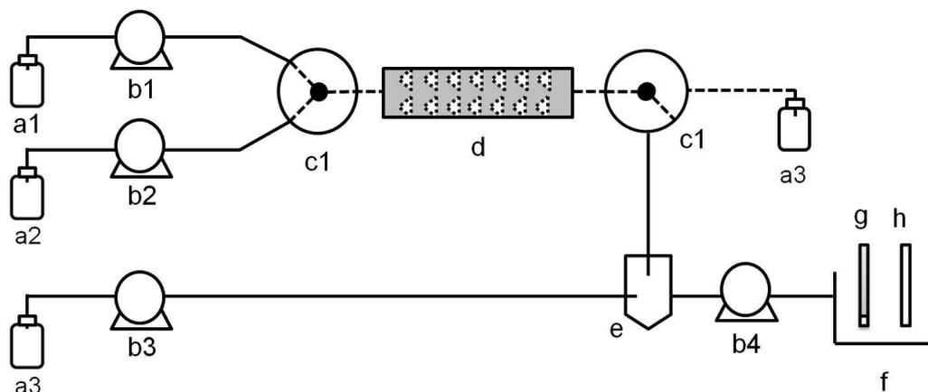
**Figure 1.** Schematic diagram of the on-line system for detection of CPF in seawater samples: (a1) conditioning solution or sample; (a2) cleaning solution or eluent; (a3) deionized water; (a4) waste; (b1), (b2), (b3), (b4) peristaltic pump; (c1), (c2) switching valve; (d) MISPE cartridge; (e) pre-concentration cell; (f) detection cell; (g) indicator electrode; (h) reference electrode
