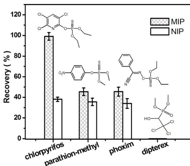
**Figure 4.** Recoveries of CPF by the MIP and NIP cartridges in the presence of parathion-methyl, phoxim and dipterex. Other conditions as in Figure 2.
