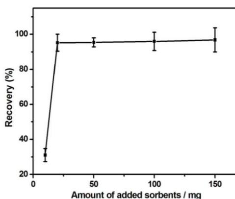
**Figure 2.** Effect of the amount of MIP sorbent on the recovery of CPF. Conditioning solution, 10 mL ACN and 10 mL deionized water; sample volume, 100 mL; washing solution, 10 mL 10<sup>-2</sup> M NaOH solution and 10 mL of deionized water; eluent solution, 10 mL ACN. Each data point represents a mean value ± relative standard deviation for three measurements.
