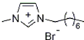
Scheme 1. Molecular structure of ionic liquid [OMIM]Br
