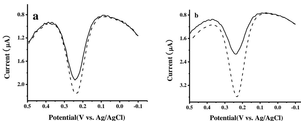
**Figure 2.** Cyclic voltammograms of PBS solution (dashed line) and 0.3 mM  $\beta$ -hydroxybutyrate (solid line) at screen printed electrode mixed with Fc-OH (a) or the mixture of Fc-OH and thionin (b).
