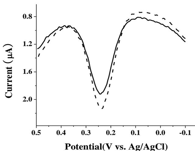
**Figure 1.** Differential pulse voltammogram (DPV) of PB solution at screen printed electrode mixed with Fc-OH (solid line) or the mixture of Fc-OH and thionin (dashed line)
