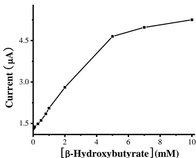
**Figure 3.** The relationship of oxidized currents with various  $\beta$ -hydroxybutyrate concentrations from 0 to 10 mM at screen printed electrode with the potential of 0.3 V.
