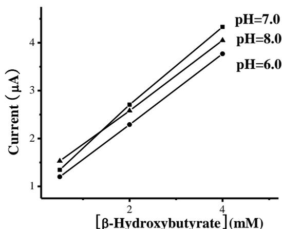
**Figure 4.** The current response of  $\beta$ -hydroxybutyrate at various pH.
