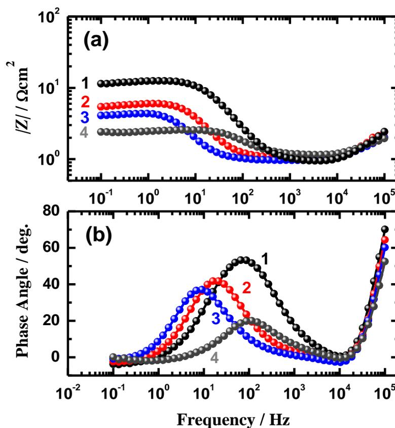
**Figure 5.** (a) Bode impedance and (b) Bode phase angle plots obtained for C-250 maraging steel electrodes after their immersion in 1.0 M H<sub>2</sub>SO<sub>4</sub> solutions for (1) 10 min, (2) 1 h, (3) 4 h and (4) 24 h at room temperature.
