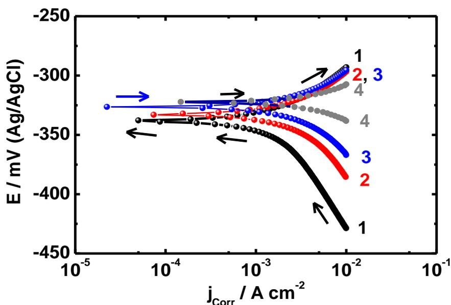
**Figure 1.** Potentiodynamic polarization curves obtained for C-250 maraging steel electrodes after their immersion in 1.0 M  $\text{H}_2\text{SO}_4$  solutions for (1) 10 min, (2) 1 h, (3) 4 h and (4) 24 h at room temperature.
