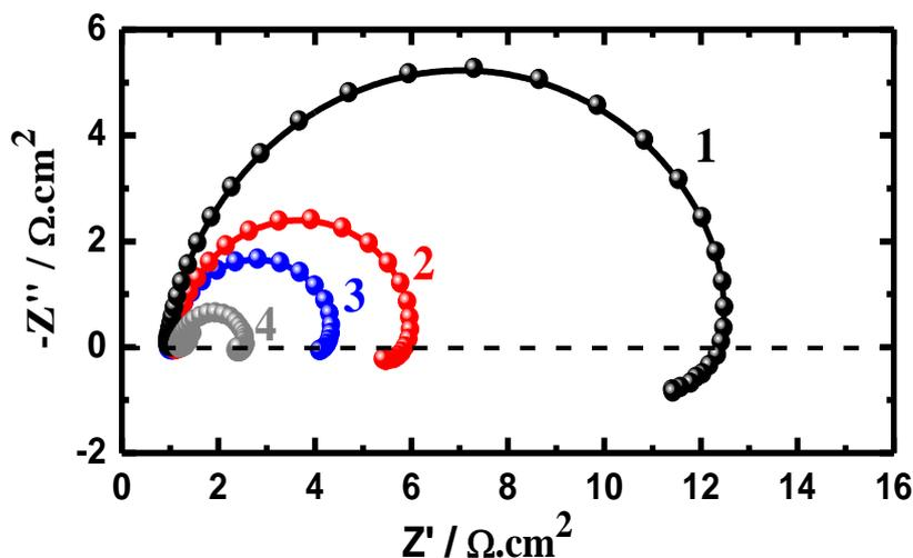
**Figure 3.** Typical Nyquist plots obtained for C-250 maraging steel electrodes after their immersion in 1.0 M  $\text{H}_2\text{SO}_4$  solutions for (1) 10 min, (2) 1 h, (3) 4 h and (4) 24 h at room temperature.
