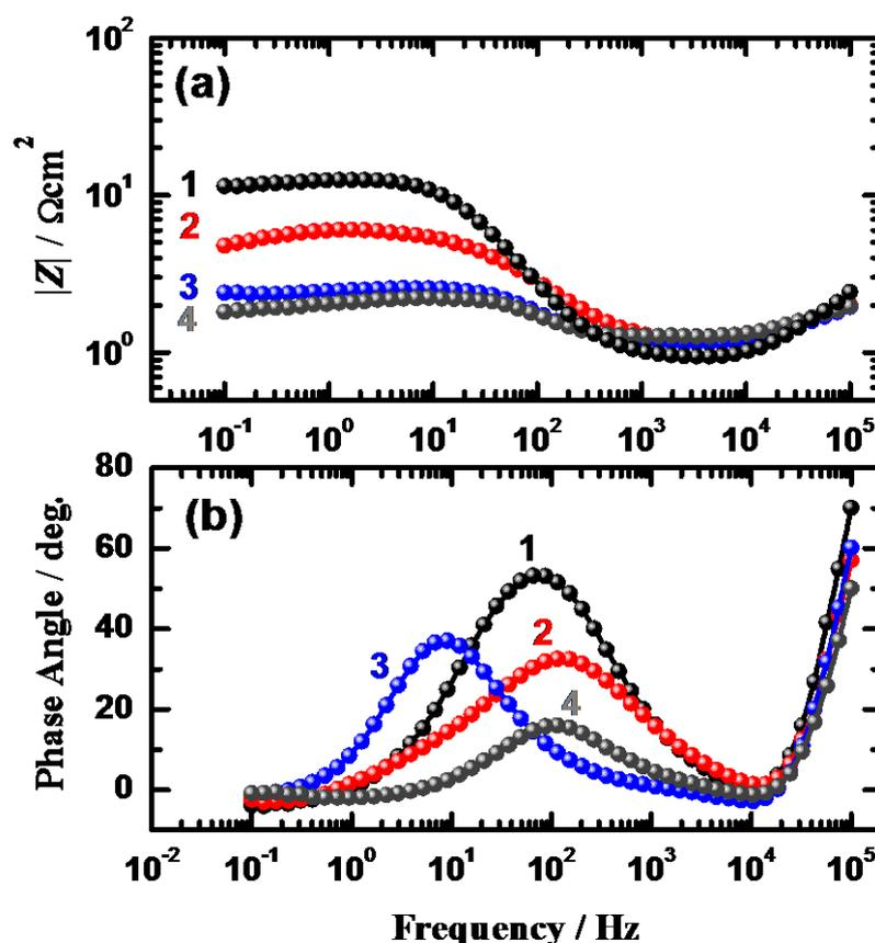
**Figure 7.** Bode impedance (a) and Bode phase angle (b) plots obtained for C-250 maraging steel electrodes after their immersion for 10 min in 1.0 M  $H_2SO_4$  solutions at (1) 20 °C, (2) 30 °C, (3) 40 °C and (4) 50 °C, respectively.
