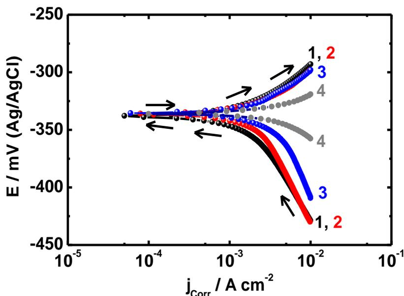
**Figure 2.** Potentiodynamic polarization curves obtained for C-250 maraging steel electrodes after their immersion for 10 min in 1.0 M  $H_2SO_4$  solutions at (1) 20 °C, (2) 30 °C, (3) 40 °C and (4) 50 °C, respectively.
