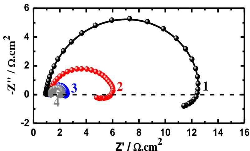
**Figure 6.** Typical Nyquist plots obtained for C-250 maraging steel electrodes after their immersion for 10 min in 1.0 M H<sub>2</sub>SO<sub>4</sub> solutions at (1) 20 °C, (2) 30 °C, (3) 40 °C and (4) 50 °C, respectively.
