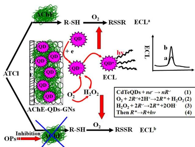
**Figure 5.** A AChE-QDs-GNs/GCE based signal-on electrochemiluminescence biosensor to detect organophosphate pesticides at AChE-QDs-GNs/GCE.
