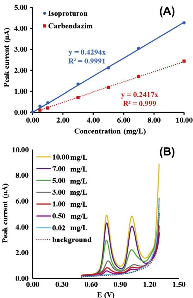
**Figure 2.** (A) Calibration curves, and (B) square wave stripping voltammetric curves for different concentrations of isoproturon and carbendazim in 1.0 M HClO<sub>4</sub>. (Reproduced with permission from ref. [24]).
