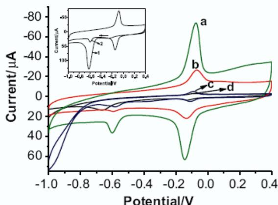
**Figure 1.** Cyclic voltammograms of MIP-IL-EGN/GCE (a), NIP-IL-EGN/GCE (b), MIP-IL-GO/GCE (c), MIP/GCE (d) in 0.1 M PBS (pH 6.8) containing 10  $\mu\text{M}$  methyl parathion (MP). Inset: the CVs corresponding to the first and second scans of MIP-IL-EGN/GCE. Scan rate: 50 mV/s. (Reproduced with permission from ref. [66]).
