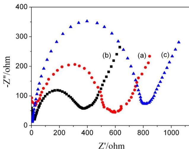
**Figure 4.** EIS (Nyquist plot) obtained at (a) bare BDD electrode, (b) Pt-CAs/BDD electrode, and (c) AChE/Pt-CAs/BDD electrode in 0.1 M KCl solution containing 0.01 M  $[\text{Fe}(\text{CN})_6]^{3-/4-}$ . Frequency range: 0.1 Hz to 10 kHz. (Reproduced with permission from ref. [28]).
