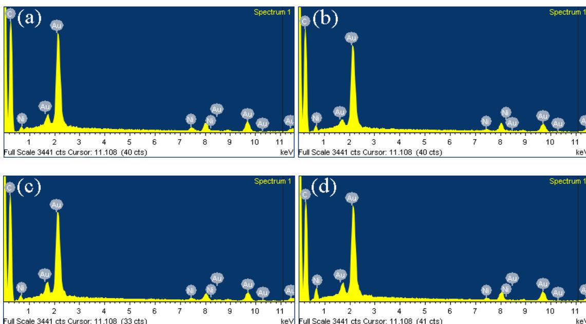
**Figure 2.** EDS spectra of the AuNi/C300 (a), AuNi/C400 (b), AuNi/C500 (c) and AuNi/C600 (d) catalysts.
