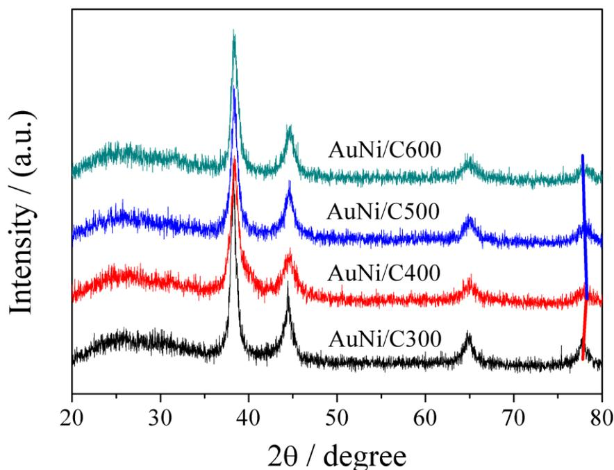
**Figure 3.** XRD patterns of the AuNi/C300 (a), AuNi/C400 (b), AuNi/C500 (c) and AuNi/C600 (d) catalysts.
