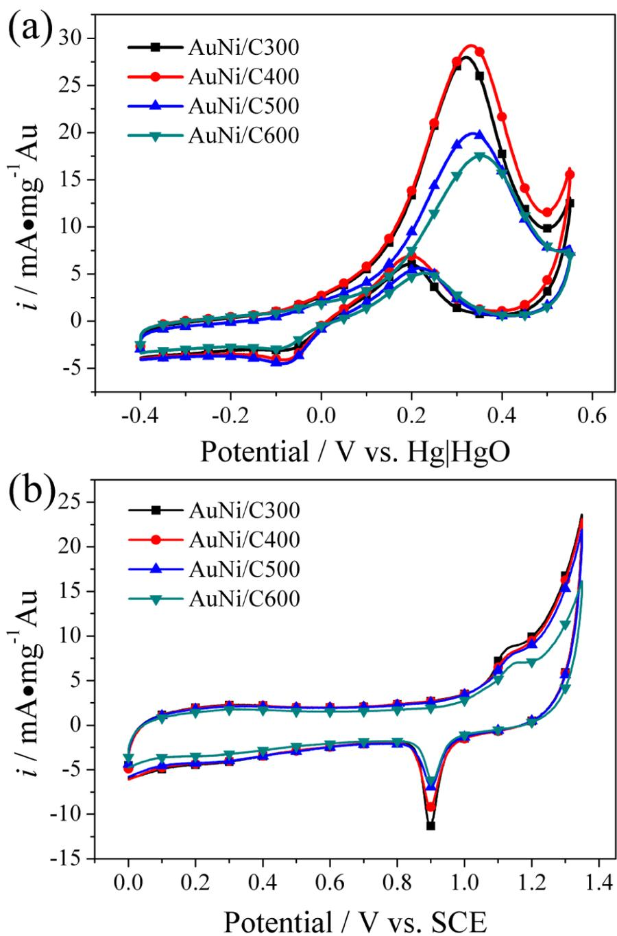
**Figure 4.** CVs on the AuNi/C catalysts at a scan rate of  $20 \text{ mV s}^{-1}$  in the deoxygenated  $0.1 \text{ M KOH} + 5 \text{ M CH}_3\text{OH}$  (a) and  $0.05 \text{ M H}_2\text{SO}_4$  (b) solutions. The species of the AuNi/C catalysts are shown in the figures.
