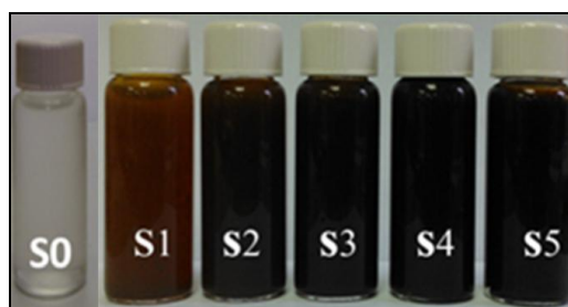
Figure 2. Photograph of [\text{Ag}(\text{Na-Alg})]^+ (S0) and [\text{Ag}(\text{Alg})] solution prepare after added of different volume of NaOH (1 M), respectively [0.5 (S1), 1 (S2), 1.5 (S3), 5 (S4) and 10 mL (S5)].
