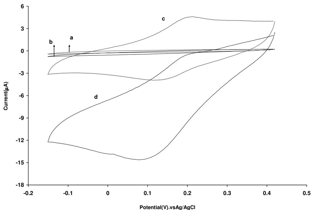
**Figure 1.** Cyclic voltammograms of thionin -MWCNTs modified GC electrode in buffer solution pH 2 at scan rate  $20 \text{ mV s}^{-1}$  in the absence (c) and presence 5.0 mM iodate (d). (a and b) as (c and d) for GC electrode modified with MWCNTs.
