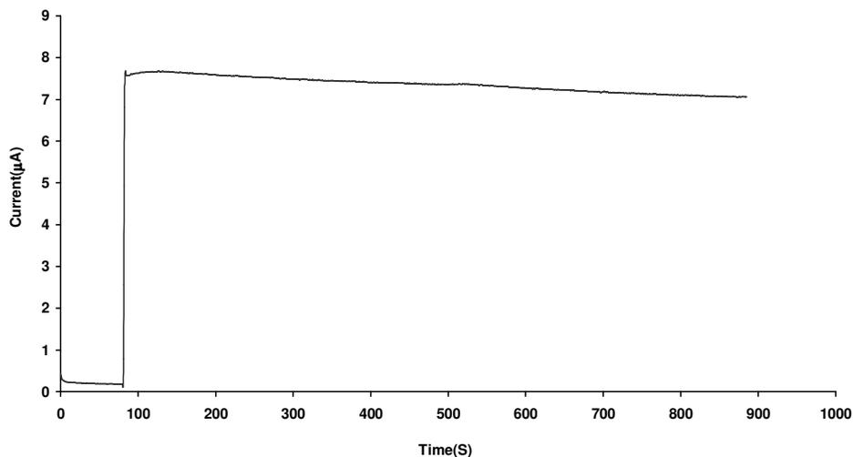
**Figure 4.** recorded chronoamperogram for 1.0 mM iodate during long period time (15 min), other condition as in Fig.3.
