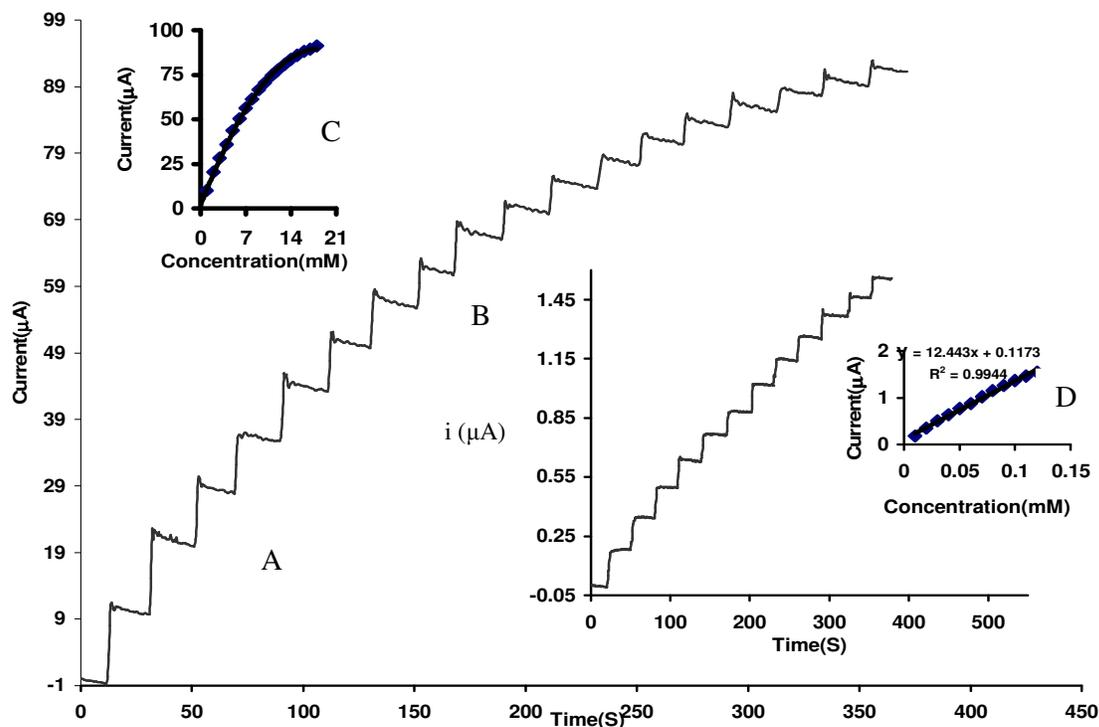
**Figure 3.** (A) Amperometric response at rotating modified electrode (rotation speed 1000 rpm) held at 0.25 V in buffer solution (pH 2) for successive addition 1 mM of periodate, (B) as (A) for 10  $\mu$ M addition. (C) Plot of chronoamperometric currents vs. periodate concentrations. (D) as (C) for lower concentration.
