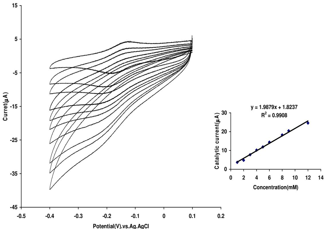
**Figure 2.** Cyclic voltammograms of thionin-MWCNTs modified GC electrode, at scan rate  $20 \text{ mVs}^{-1}$  with increasing periodate concentration (from inner to outer) 0.0, 1.0, 2, 3, 4, 5, 6, 8, 9 and 12 mM of periodate in pH 7 phosphate buffer solution. Inset, plot of peak current vs. periodate concentrations.
