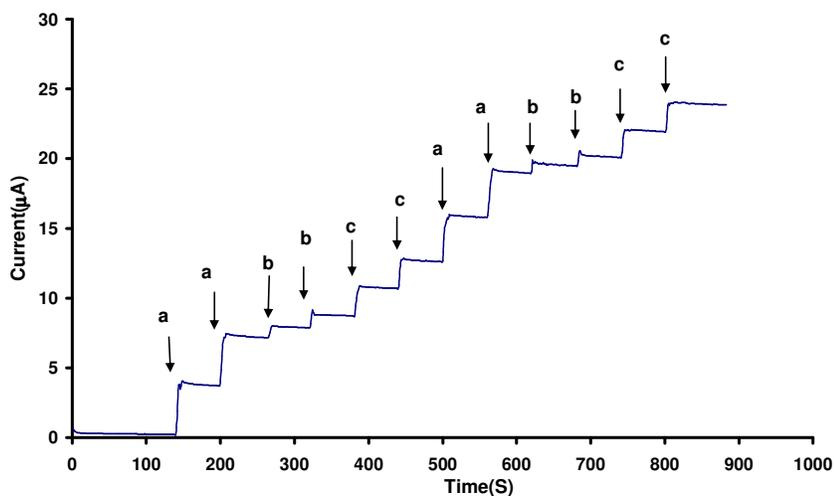
**Figure 5.** Steady- state current response obtained for reduction of periodate ,iodate and nitrite at thionin-MWCNTs modified GC electrode in pH 2 upon the injection of (a) and (c) 0.5 mM of periodate and iodate, (b) 2mM of nitrite, other conditions as in Fig. 3.
