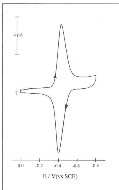
**Figure 2.** Cyclic voltammograms of a BPG surface adsorbed by  $8.9 \times 10^{-10} \text{ mol.cm}^{-2}$  of ACAE in electrolyte: 0.1 M  $\text{Na}_2\text{SO}_4$  + 0.1 M  $\text{CH}_3\text{COOH}/\text{CH}_3\text{COONa}$  (pH 5.8). Potential scan rate:  $100 \text{ mV.s}^{-1}$
