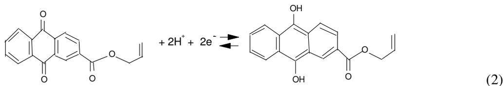
The attachment of adsorbed ACAE coating on the graphite electrode is stable. The coated electrode can be scanned between 0 and  $-0.8 \text{ V}$  in a pH 5.6 solution for 4 hours without apparent decrease in the magnitude of the peak current of the wave near  $-0.4\text{V}$ .
