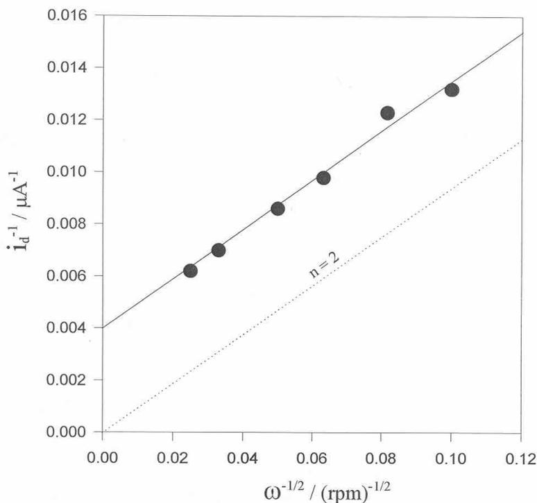
**Figure 7.** Koutecky-Levich plot for data in Figure 6. The dashed line corresponds to the calculated response for the diffusion-convection-controlled curve for two-electron reduction of  $O_2$ .
