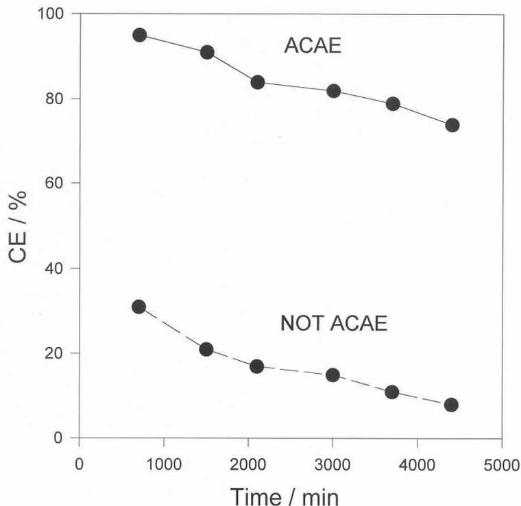
**Figure 8.** The current efficiencies of a three-day run. The data were obtained with a BPG electrode ( $0.79 \text{ cm}^2$ ) coated with  $1.1 \times 10^{-9} \text{ mol.cm}^{-2}$  of ACAЕ (upper curve), and the same electrode but without catalyst (bottom curve), rotated at 400 rpm, in  $1.3 \times 10^{-3} \text{ M O}_2$  solution (pH5.6). Supporting electrolyte as in Figure 2. Current density of electrolysis:  $160 \mu\text{A.cm}^{-2}$ .
