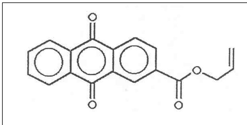
**Figure 1.** Structure of anthraquinone-2- carboxylic-allyl ester (abbreviated as ACAE).
