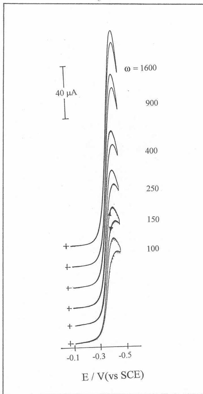
**Figure 6.** Electroreduction of  $1.3 \times 10^{-3}$  M O<sub>2</sub> on a rotating BPG electrode coated with  $1.0 \times 10^{-9}$  mol.cm<sup>-2</sup> of ACAE. The electrode rotating rates: (a) 100 rpm; (b) 150 rpm); (c) 250 rpm; (d) 400 rpm; (e) 900 rpm; and (f) 1600 rpm. Supporting electrolyte as in Figure 1 (pH5.6). Potential scan rate: 10 mV.s<sup>-1</sup>.
