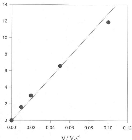
**Figure 3.** The scan rate dependence of the average of the anodic and cathodic peak currents on cyclic voltammograms as in Figure 2.
