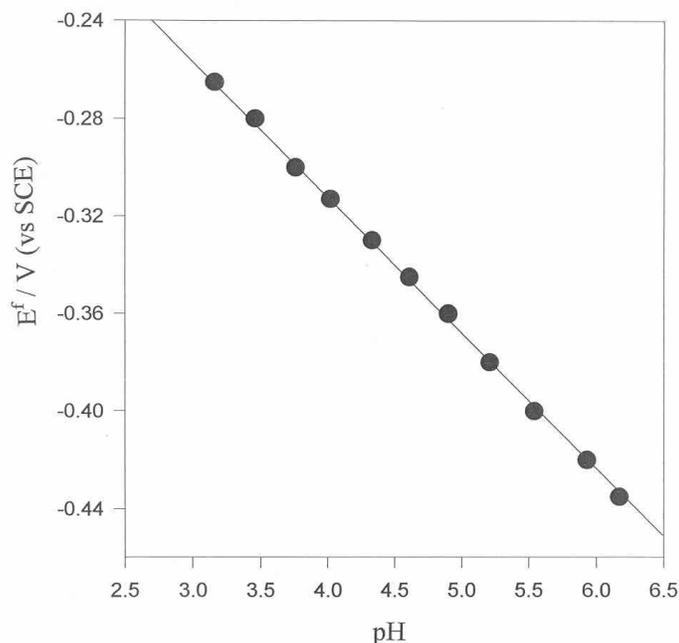
**Figure 4.** The pH dependence of the formal potential of the wave in Figure 2 estimated by averaging the anodic and cathodic peak potentials. Electrolytes as in Figure 2. Potential scan rate:  $20 \text{ mV}\cdot\text{s}^{-1}$ .
