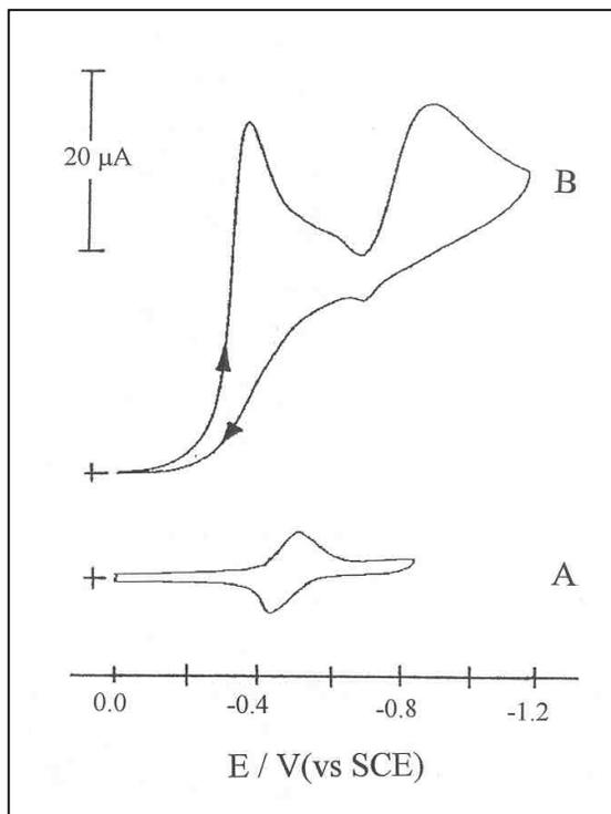
**Figure 5.** Cyclic voltammograms of a BPG electrode coated with  $9.0 \times 10^{-10}$  mol.cm<sup>-2</sup> of ACAE in pure supporting electrolyte (a), and  $1.3 \times 10^{-3}$  M of  $O_2$  (b). Supporting electrolyte as in Figure 2 (pH 5.6). Potential scan rate:  $10 \text{ mV} \cdot \text{s}^{-1}$ .
