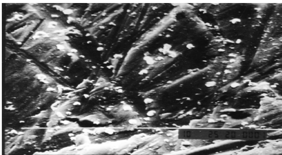
Figure 6. SEM of the 316L SS surface after potentiodynamically treated in 0.5 M NaCl + 0.001 M MBI solution.
